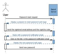
Fig. 2. Sequence diagram for the Netml password reset system
