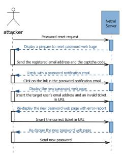
Fig. 3. Sequence diagram for the Netml password reset system under attack
