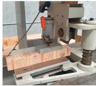
Figure 6. Shear test setup.
