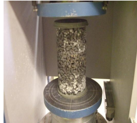
Figure 1. Compressive strength testing rig
