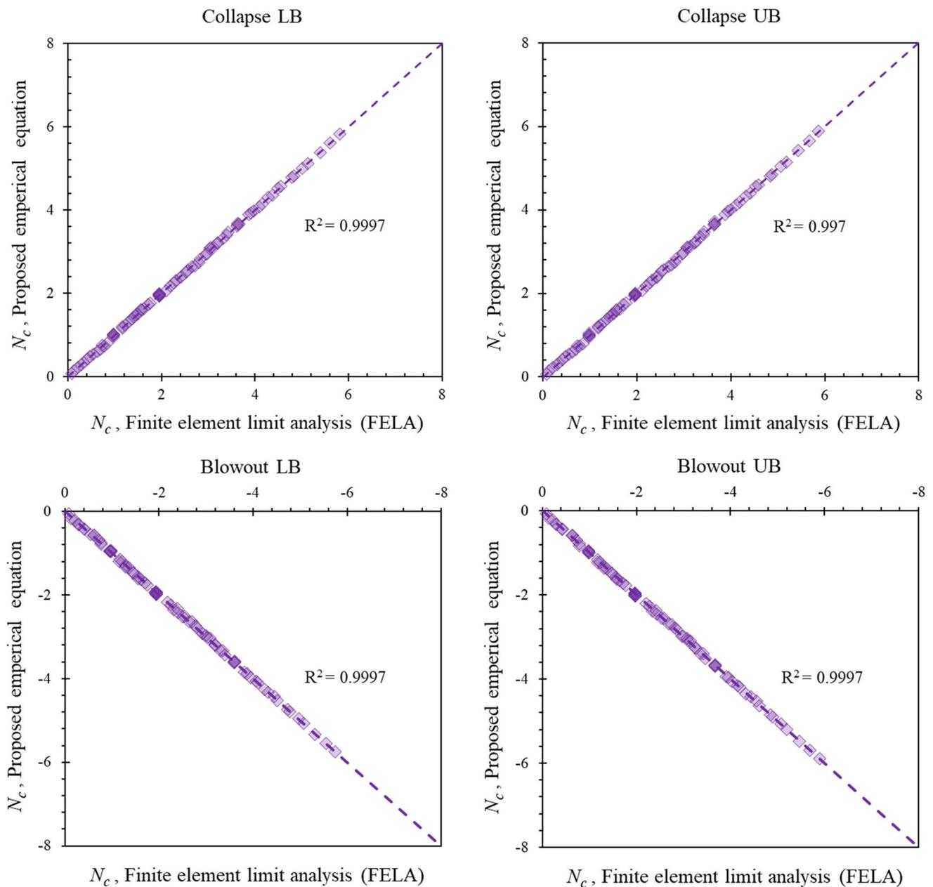
**Fig. 13** Comparison of results– the finite element analysis and the proposed equation
