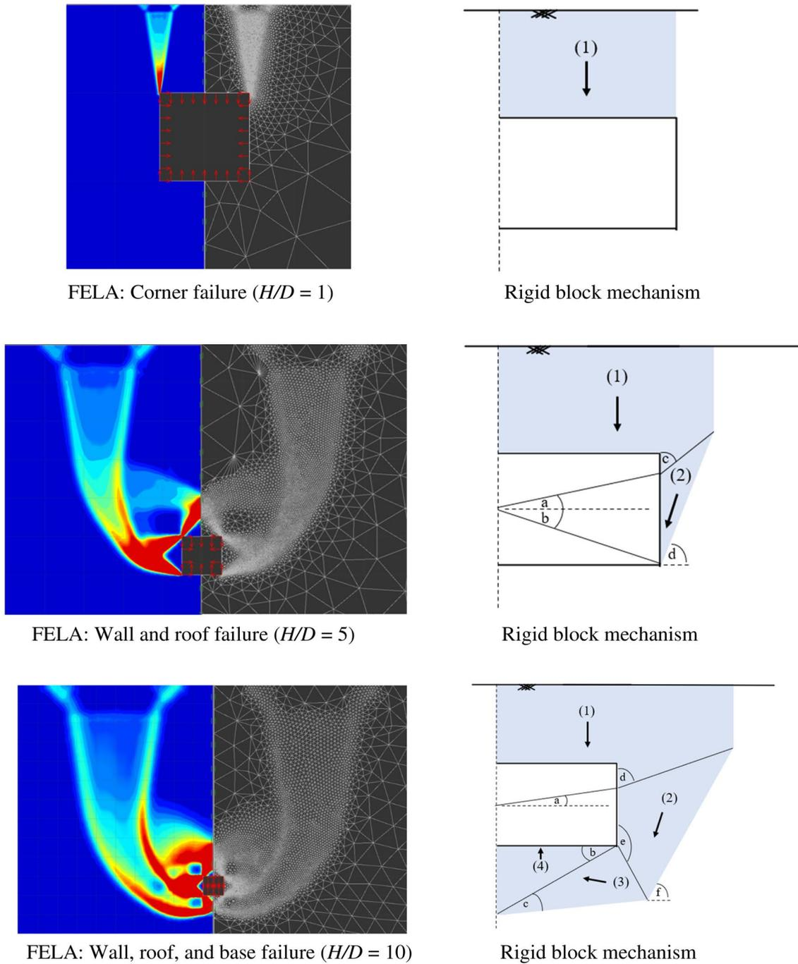
**Fig. 5** Failure mechanisms (LHS) and final adaptive mesh (RHS) for  $B/D=1$
