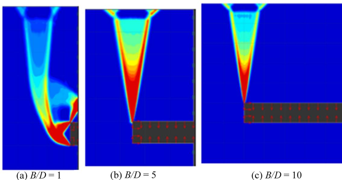
Fig. 7 Failure mechanisms for  $H/D=7$
