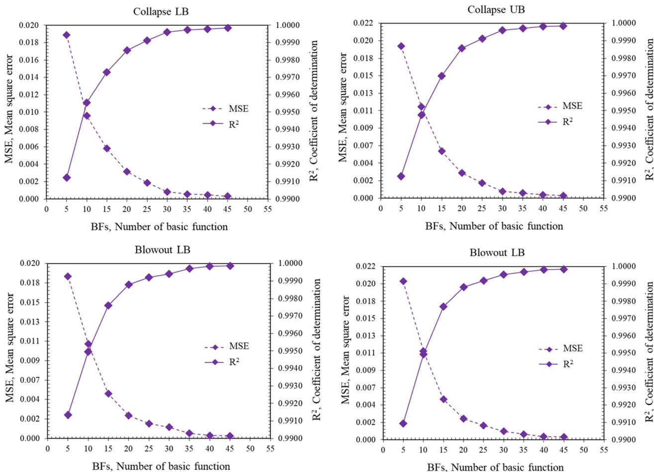
Fig. 11 Effect of number basic functions on  $R^2$  and mean square error (MSE)
