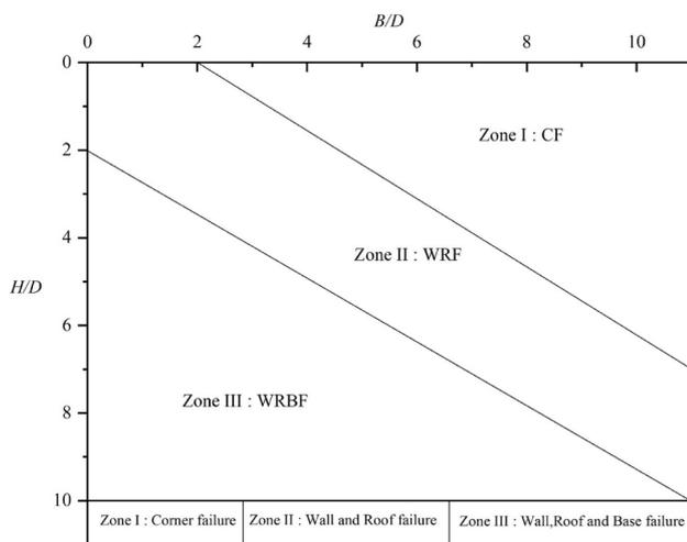
Fig. 9 Summary of all failure mechanisms
