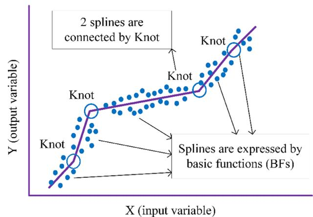
Fig. 10 Illustration of MARS model process
