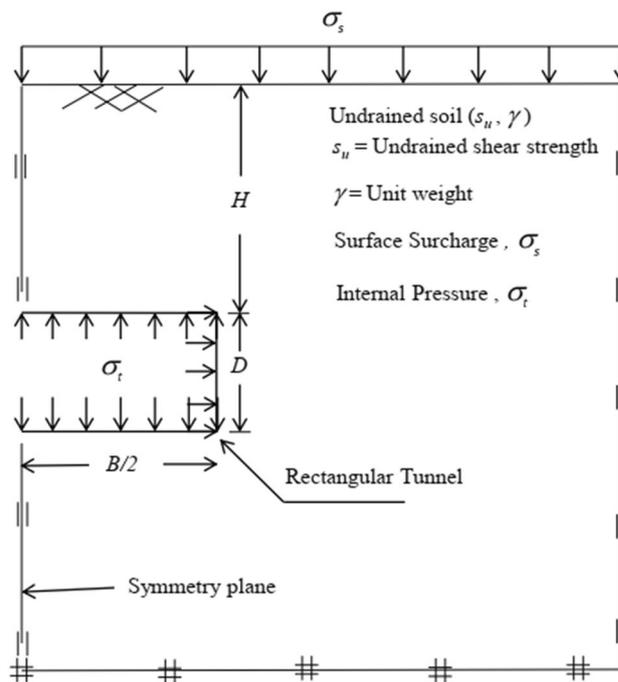
Fig. 1 Rectangular tunnel in symmetry condition-problem definition
