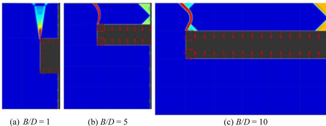
Fig. 6 Failure mechanisms for  $H/D=1$
