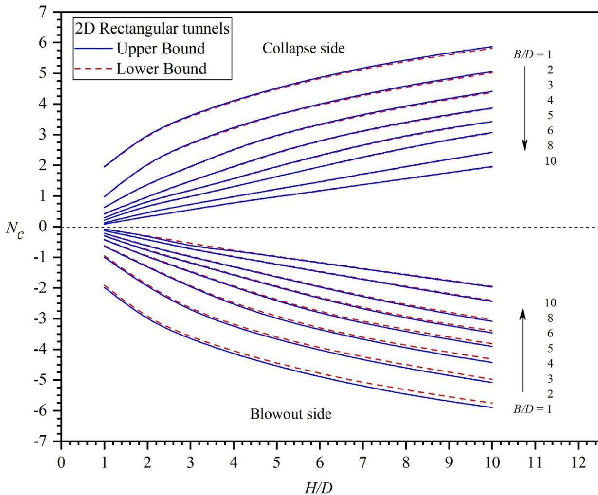
**Fig. 4**  $N_c$  results for collapse and blowout ( $H/D=1-10$ ,  $B/D=1-10$ )
