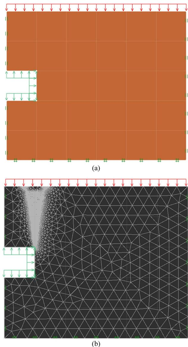
Fig. 2 a Numerical model and b Typical adaptive mesh
