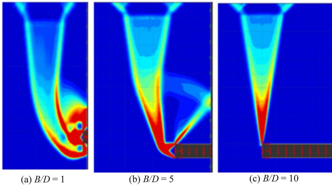
Fig. 8 Failure mechanisms for  $H/D=10$
