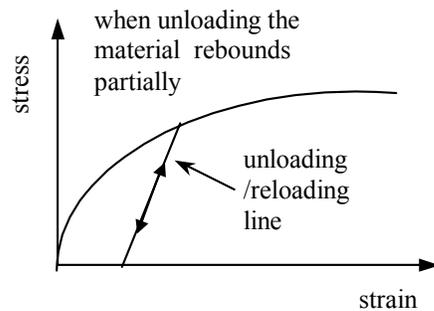
**Figure 2.** Stress-strain relationship for an elasto-plastic material.
