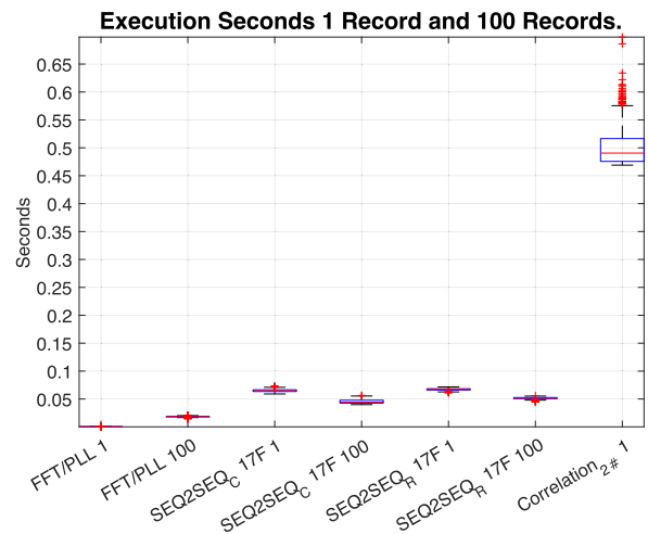
FIGURE 7. Execution speed of the simpler FFT/PLL method is faster in comparison to the deep network model which performs well on larger batches and is faster than the brute force cross-correlation method.
