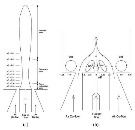
Figure 5. Schematic diagrams for bluff-body burner, (a) flame flow field with central fuel jet and annulus air co-flow, (b) flame re-circulation zone .
