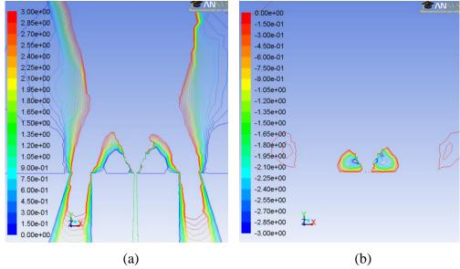
Figure 4. Contour of Y velocity, (a) 0 to 3.0 m/s, (b) -3.0 to 0 m/s.
