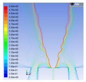
Figure 3. Contour of total velocity magnitude (0 to 5.0 m/s)
