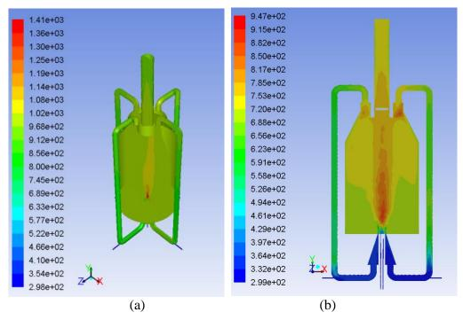
Figure 1. Early stage of the of combustion process in open furnace, not MILD combustion state yet, (a) 3D image, (b) 2D image
