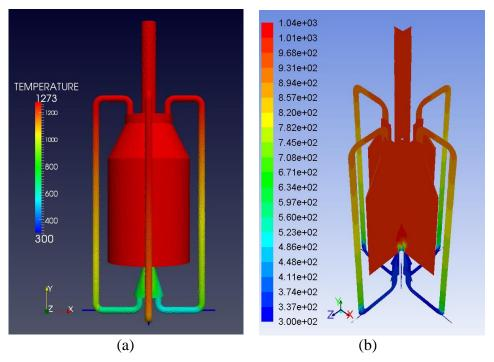
Figure 2. MILD combustion state was achieve, (a) furnace wall temperature at 1273 K, (b) inside chamber temperature 1040 K
