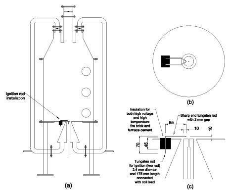
Figure 6. Schematic diagrams of combustion chamber, (a) ignition rod location, (b) location plan view and (c) location side view of ignition location and installation
