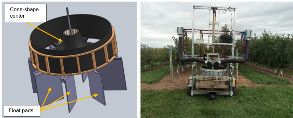
Figure 10. A low-cost apple harvest-assist unit (right) mounted with a bin filler (left) (Zhang et al., 2014, 2016a).
