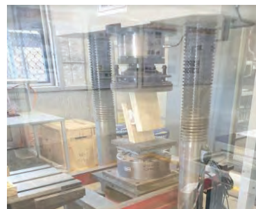
Figure 1. Two plate shear test set-up
