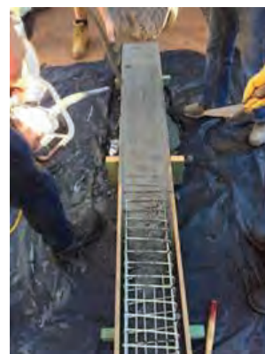
Figure 1 – Casting a Portland concrete railway sleeper designed with GFRP bars
