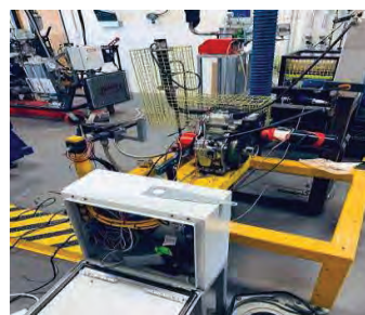
Fig. 1–The Yanmar L48N engine stand, available at USQ within cylinder during run, and composition of exhaust gas emissions will be collected.
