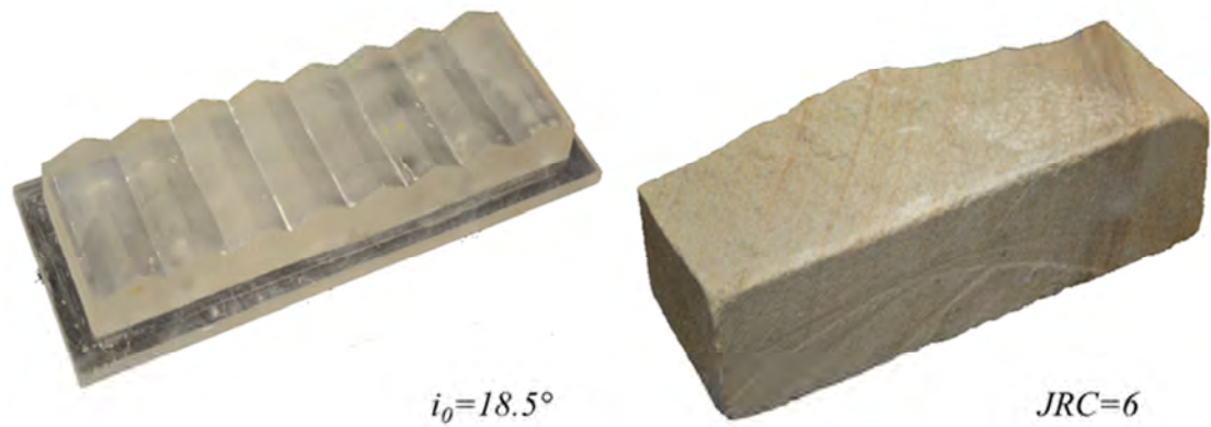
Figure 4-1 [left] Mould of Type II asperity surface, [right] Field sample
