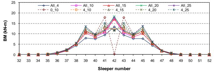
Figure 4. Maximum bending moment in sleepers 32 to 52.
