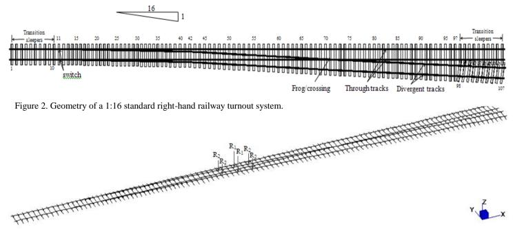
Figure 3. Grillage beam model for 1:16 standard right-hand railway turnout.
