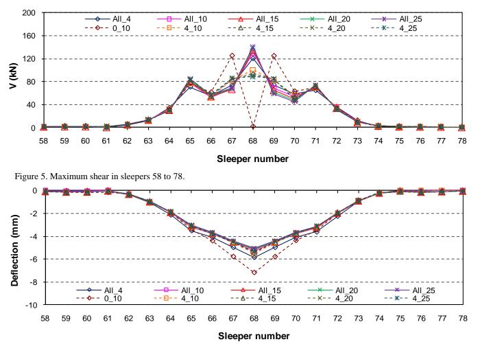
Figure 6. Maximum vertical deflection in sleepers 58 to 78.
