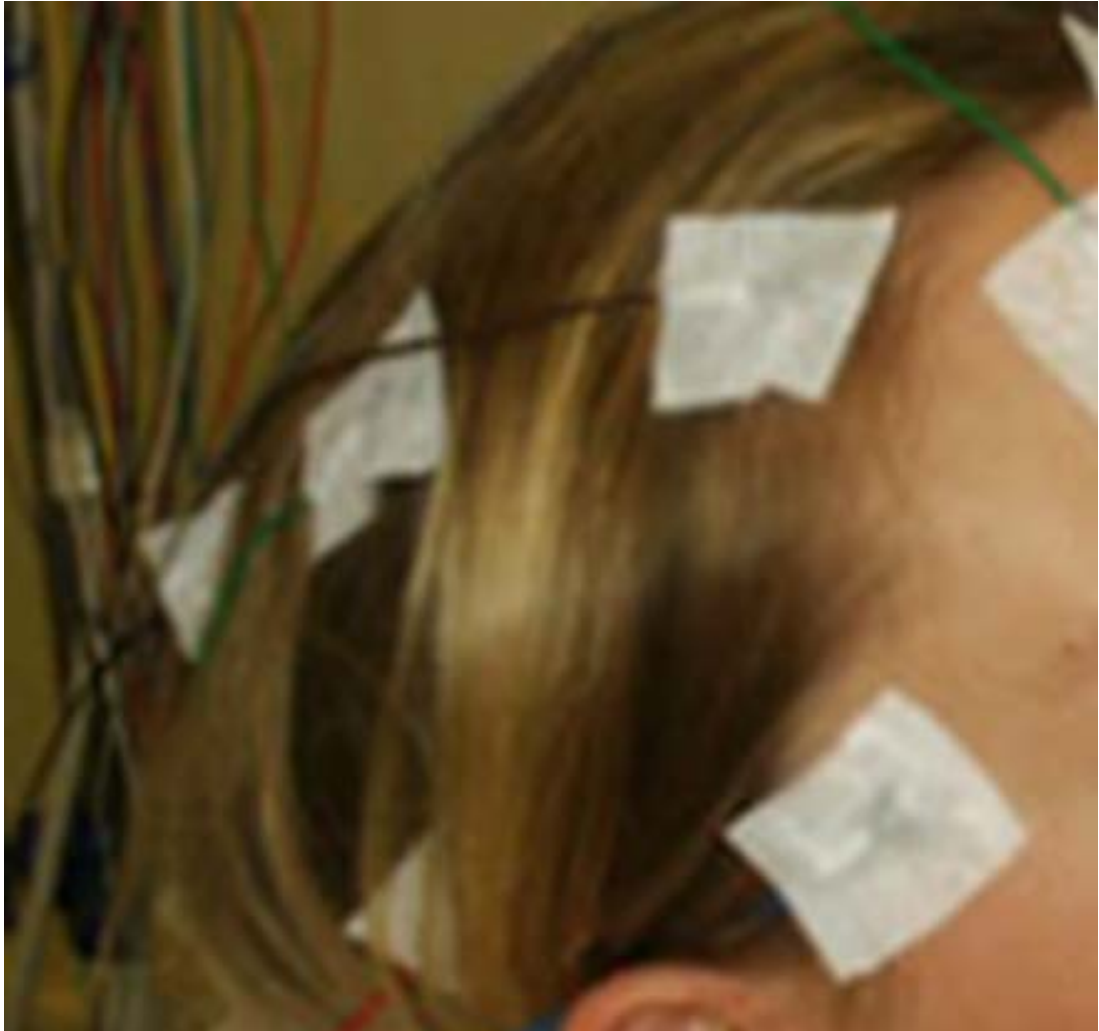
Figure 4-12 Subject with 10mm gold capped electrodes fitted to the scalp
