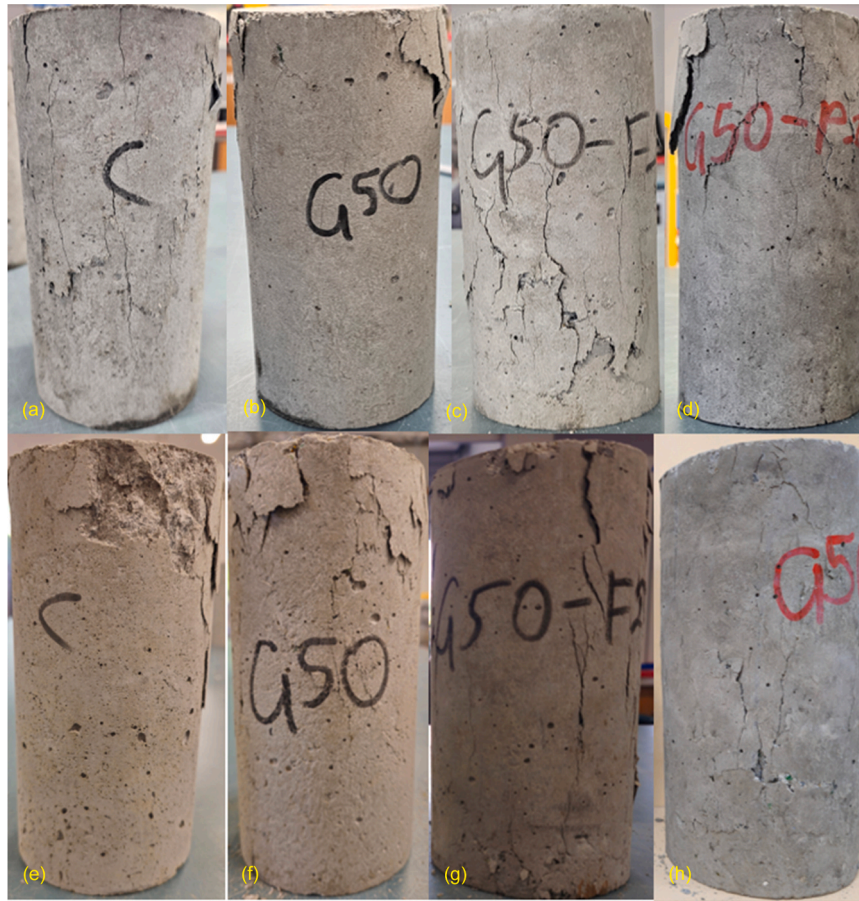
Fig. 10. Failure modes of tested cylinders for compression: 28-day cylinders; (a) 0 GFA-0FA-0PA, (b) 50GFA-0FA-0PA, (c) 50GFA-20FA-0PA, (d) 50GFA-0FA-20PA, and six-month cylinders; (e) 0GFA-0FA-0PA, (f) 50GFA-0FA-0PA, (g) 50GFA-20FA-0PA, (h) 50GFA-0FA-20PA.
