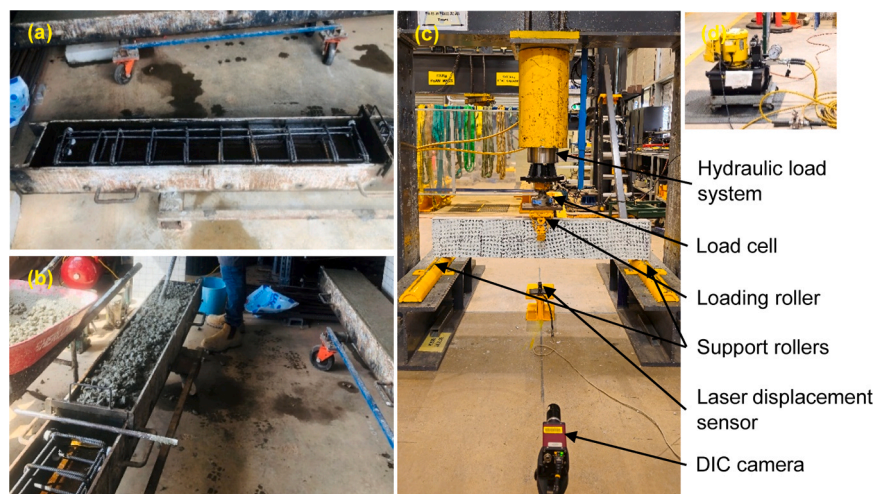
Fig. 4. (a) steel reinforcement cage inside the formwork; (b) concrete pouring and compaction; (c) Load setup and instrumentation; (d) hydraulic pump unit.
