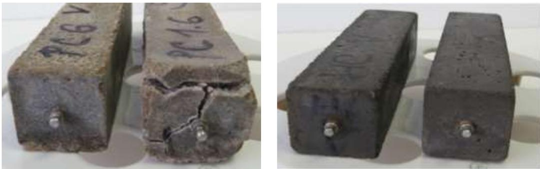
(a) OPC mortar immersed 4 years in Na<sub>2</sub>SO<sub>4</sub> (b) HAC mortar immersed 5 year in Na<sub>2</sub>SO<sub>4</sub>
