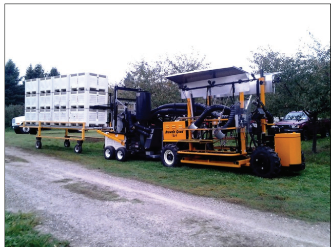
Figure 4. DBR vacuum harvest-assist platform (PBW, 2016).
