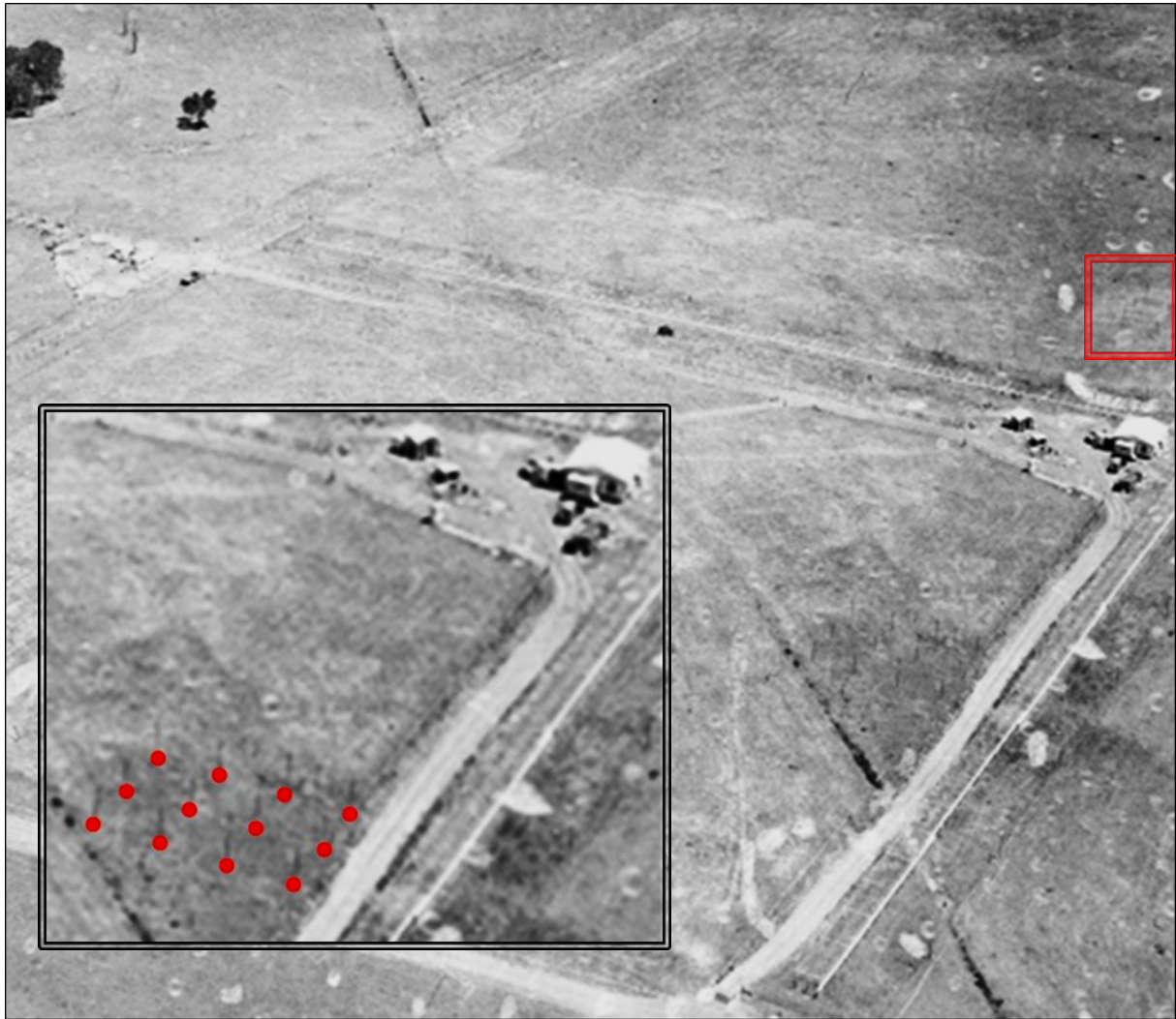
Figure 11: An aerial photograph 10 of Fleurs field station taken on 22 February 1956 showing the Chris Cross receiver hut (upper left), the Chris Cross under construction, the southern and eastern arms of the Mills Cross and the Mills Cross receiver hut (extreme right). The large inset shows a close-up of the eastern element of the 19.6 MHz interferometer and the Mills Cross receiver hut, with the bases of the poles that supported the four dipoles marked with red circles. Within the red box are what appear to be some of the poles associated with the western element of the interferometer (CRAIA, B3923-14; photograph modifications: Wayne Orchiston).
