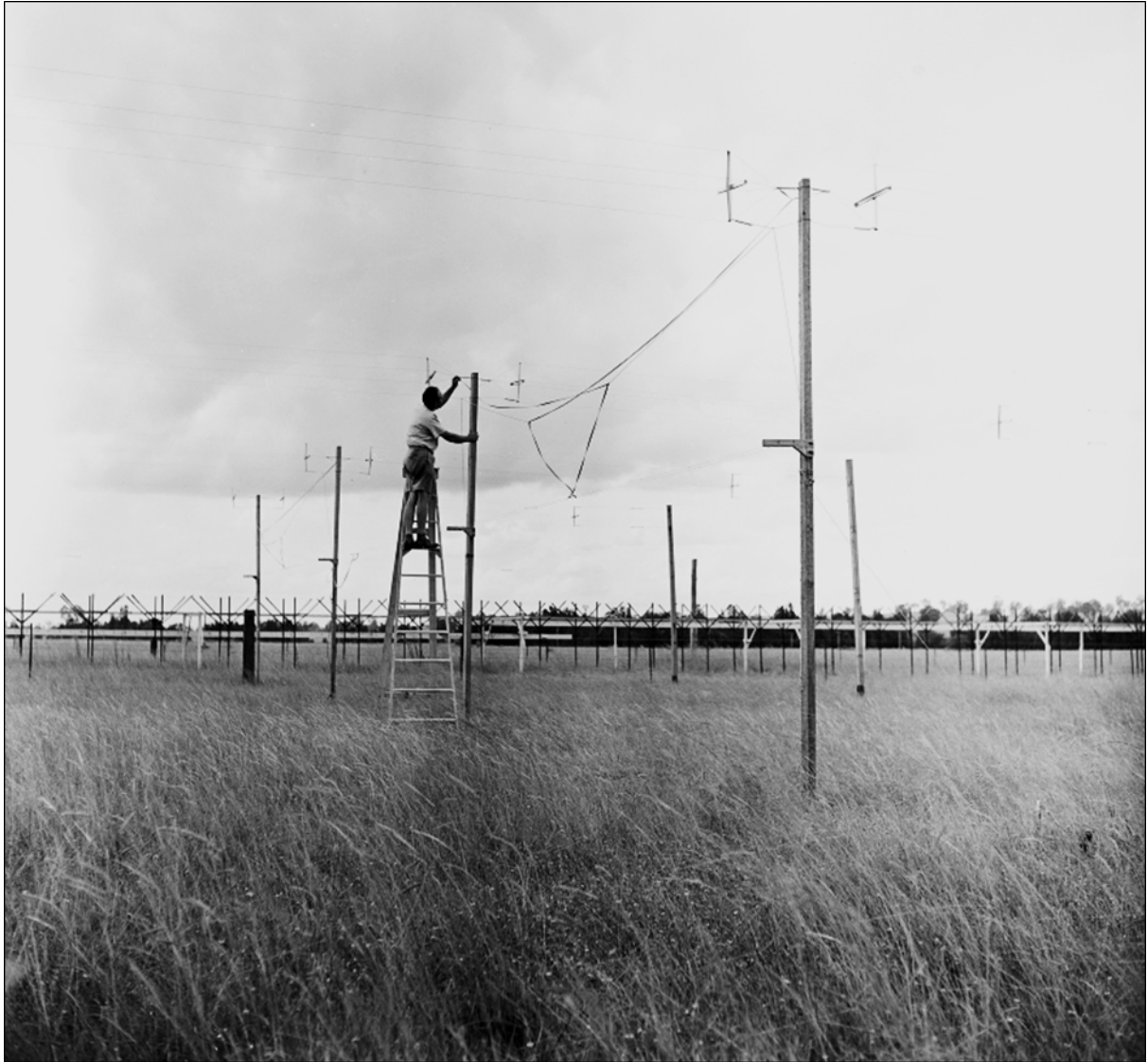
Figure 8: This 22 February 1956 photograph shows one of the low-frequency radio telescopes at Fleurs used for observations of Jupiter in 1955–1956. The array was erected just south of the eastern arm of the Mills Cross. The presence of four sets of poles (with no indication that the array extended to eight dipoles) suggested that this was either the 14 MHz array or one of the 19.6 MHz interferometer elements. Note that the poles are aligned perpendicular to the Mills Cross (which is in the background), with the low frequency dipoles running E-W (courtesy: CRAIA, B3932-14).
