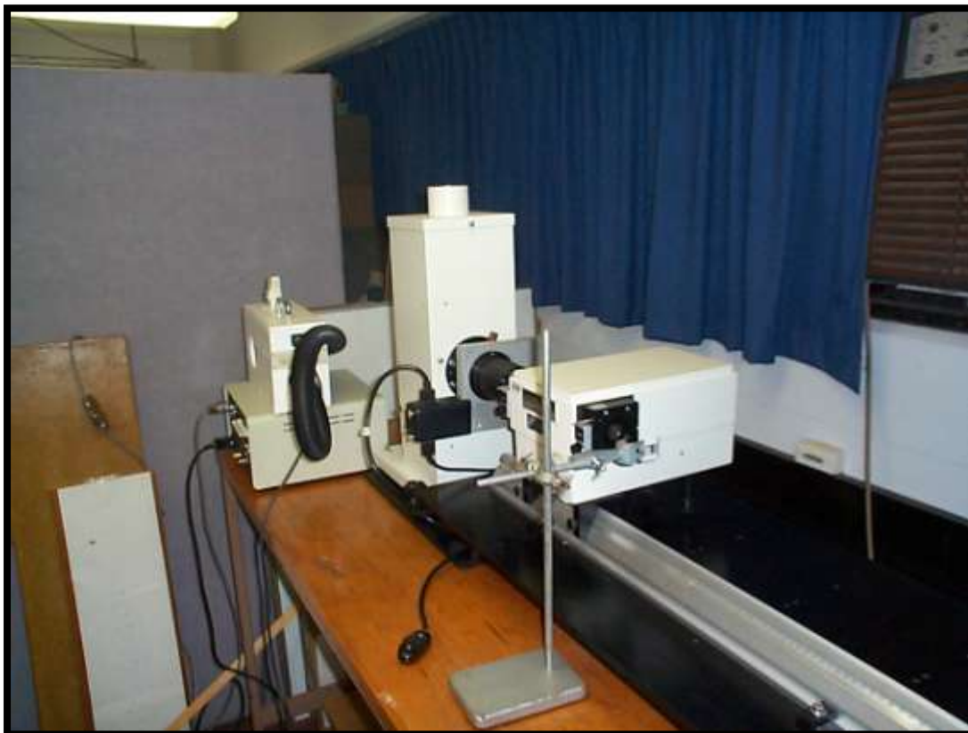
Figure 6.3: The irradiation monochromator at the University of Southern Queensland's physics laboratory. The lamp housing is seen toward the rear of the instrument and the monochromator is toward the front. A PPO film actinometer is held in front of the output aperture by a retort stand for irradiation with monochromatic UV.
