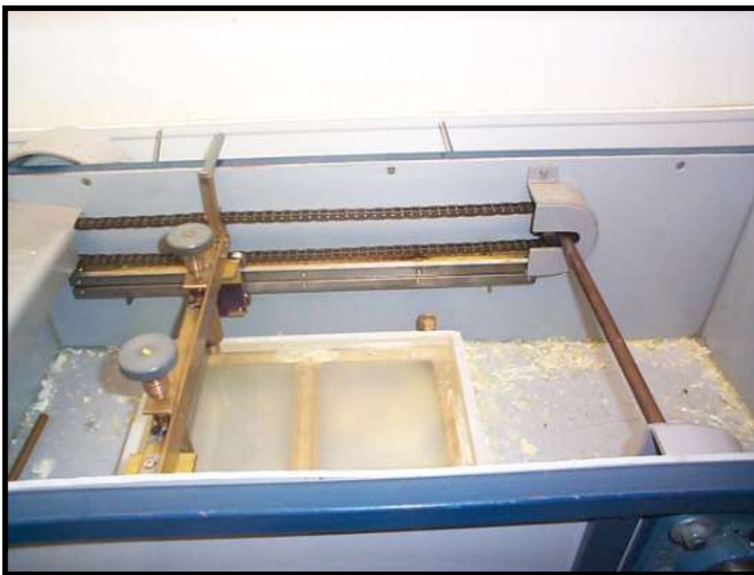
Figure 6.1: The polymer film casting table employed by physicists at the University of Southern Queensland for the fabrication of various chemical films for use in UV actinometry.
