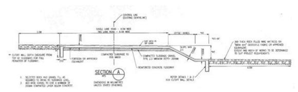
Figure 1 Cross section of floodway Type 2
