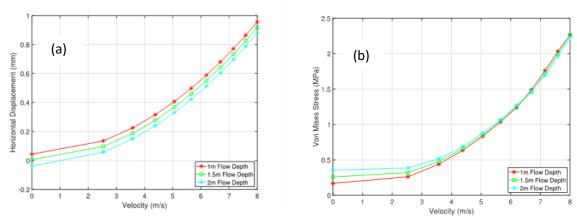
Figure 4 Horizontal displacement and Von Mises stress with increasing flow depth and velocity
