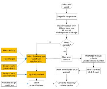
Figure 8 Floodway design process
