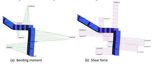
Figure 7 Sample of 2D frame model for M\* and V\* distribution
