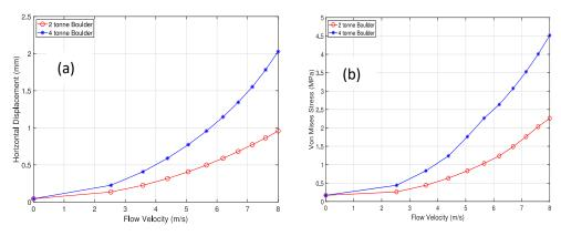
Figure 5 Effect of 2 and 4 tonne boulder impact
