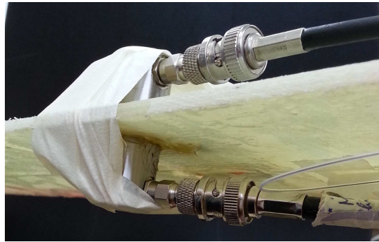
Figure 5.48: Example of piezoelectric sensors' mounting.
