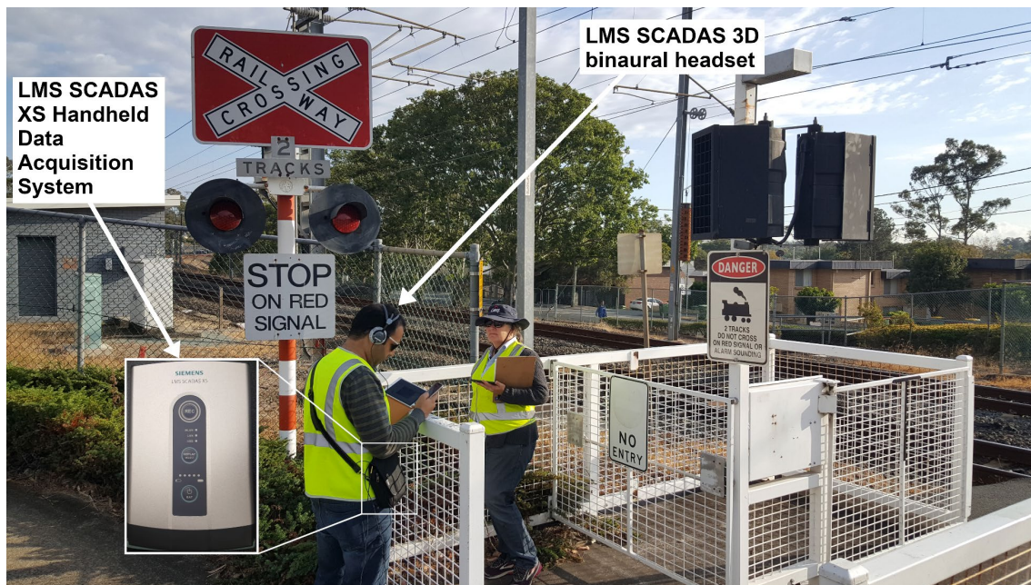
Figure 2: Siemens LMS SCADAS 3D binaural headset and the LMS SCADAS XS Handheld Data Acquisition System as used during observations.
