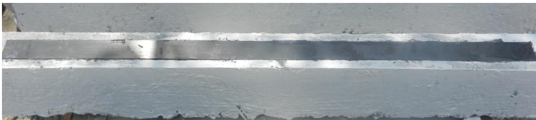
Fig. 4. CFRP bonded externally to RC beam
