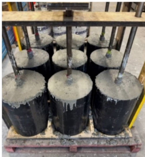
(c) Concrete pouring process
