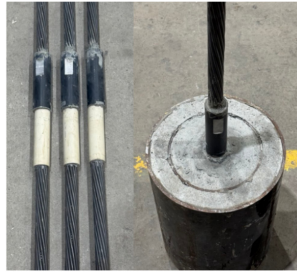
Fig. 8. The details of the cable bolt encapsulation (a), and a view of the prepared samples (b).
