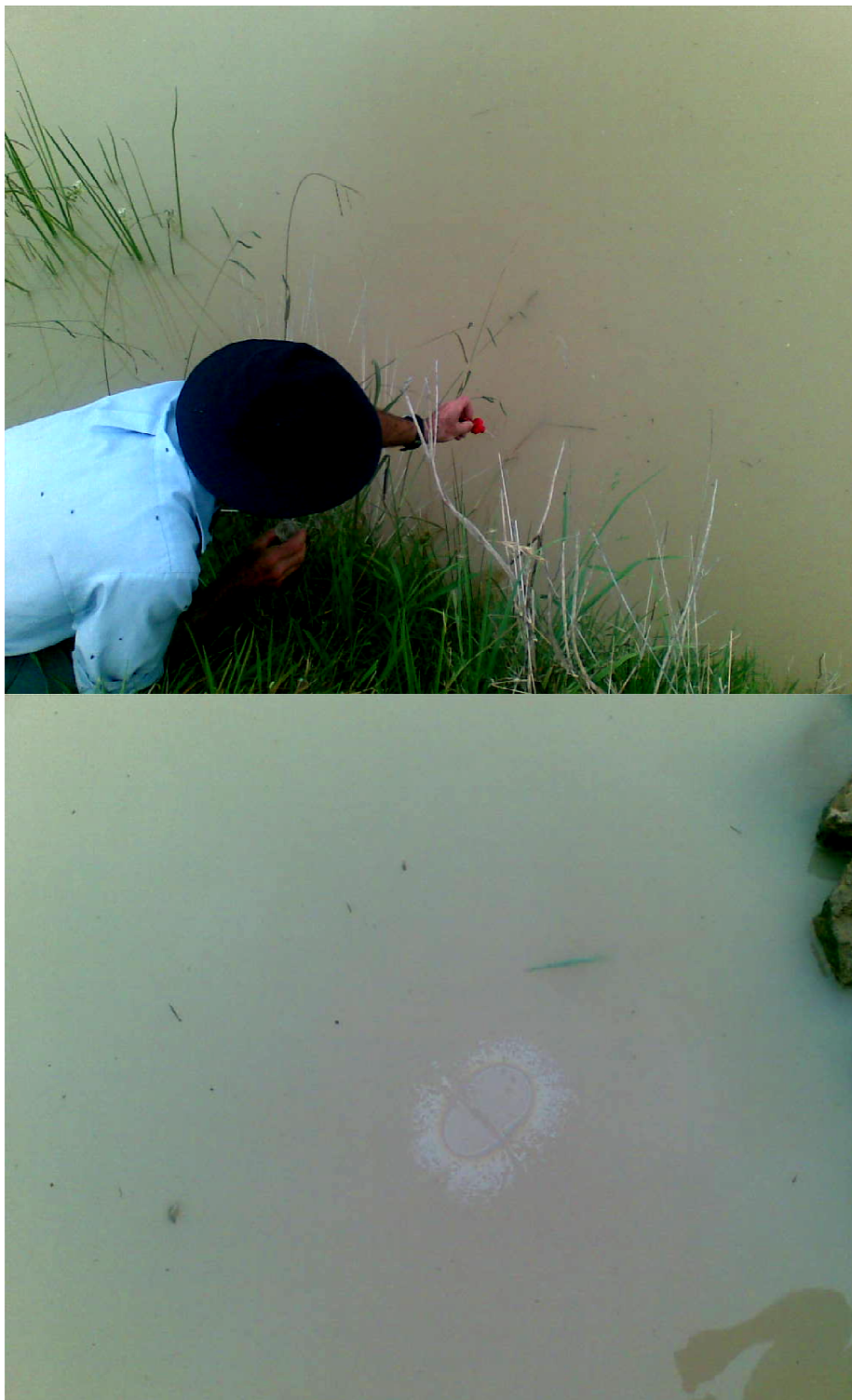
Figure 2.24 Testing for monolayer presence using indicator oils (Albrecht, 2011)
