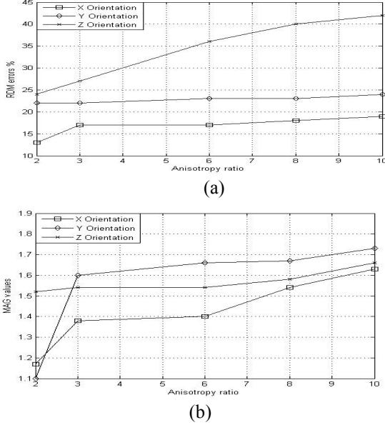
**Fig. 4 RDM and MAG errors for different WM anisotropy ratio on X, Y and Z orientations in Head model C using longitudinal conductivity. (a) Anisotropy ratio vs RDM errors and (b) Anisotropy ratio vs MAG values.**
