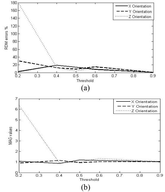
**Fig. 2 RDM and MAG errors produced by reference model and anisotropic model generated by WM anisotropic conductivity using Head model A. (a) presents RDM errors against thresholds and (b) shows MAG values vs thresholds.**
