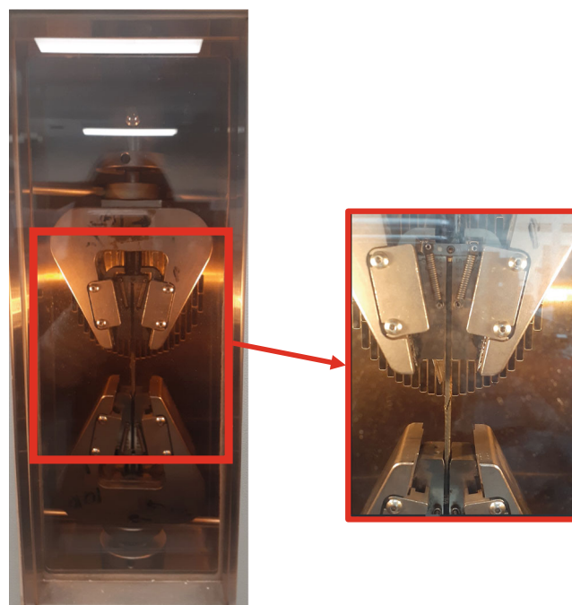
FIGURE 3 Experimental setup for tensile test at high temperatures.
