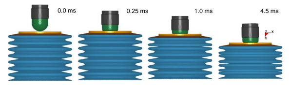
Figure 3: Stages of the projectile P2 and the surrogate MTHOTA during the impact
