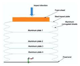
Figure 1: Cross section of the MTHOTA FE model thorax surrogate
