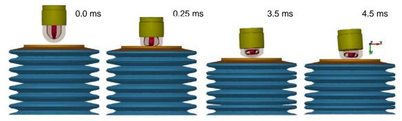
**Figure 6:** Stages of P1 projectile with 2.0 mm thick foil and the surrogate during the impact
