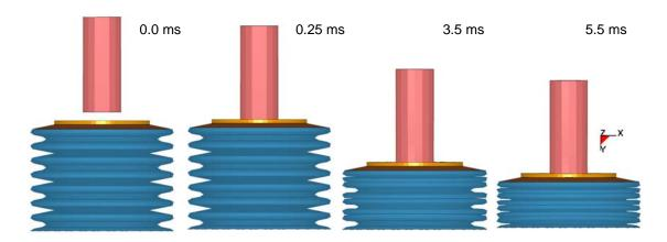
Figure 4: Stages of the projectile P3 and the surrogate MTHOTA during the impact
