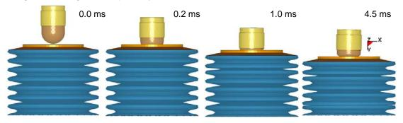
Figure 2: Stages of the projectile P1 and the surrogate MTHOTA during the impact
