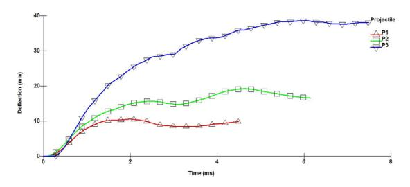
Figure 5: Relative deflection of the impact plate with respect to the plate-3
