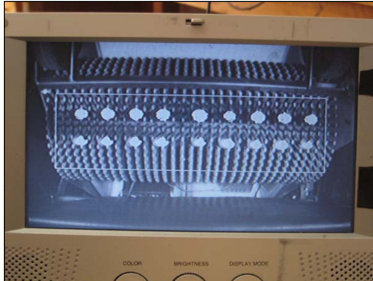
Figure 7. Typical nut detection results using FPGA colour analysis. The rectangle outline on the pinwheel is the region of interest that was analysed for nut detection. Detected nuts are overlaid with filled ellipses.
