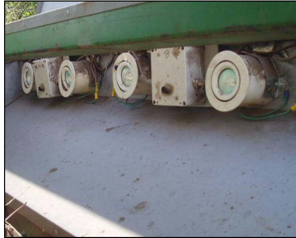
Figure 4. Two (of three) embedded systems on the tractor-mounted harvester. Each system consisted of a microprocessor, camera and two halogen lights.
