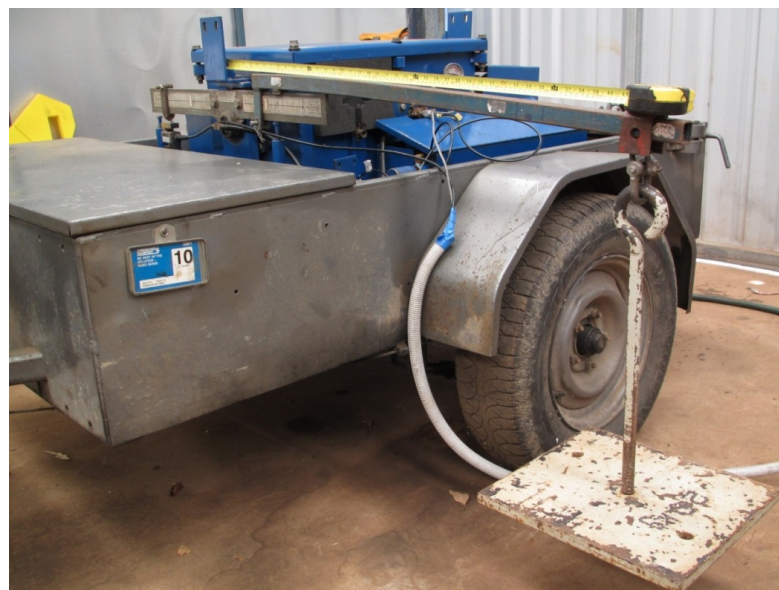
Figure 3.5: Torque calibration for the load-cell.
