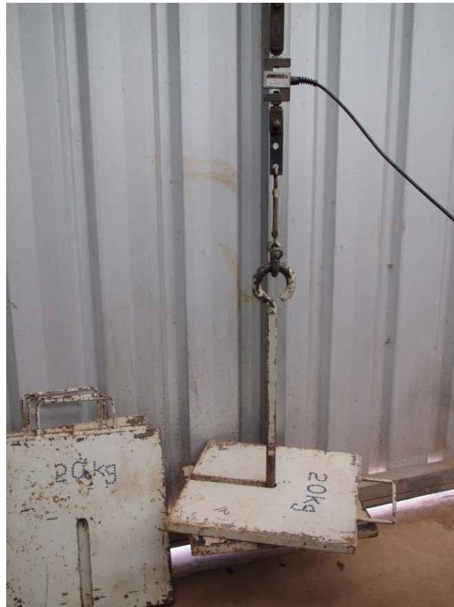
Figure 3.6: Direct force load-cell calibration.
