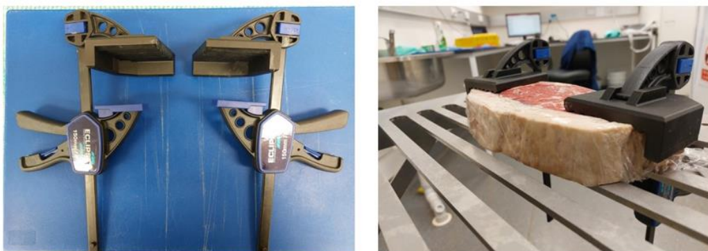
Figure 32: The trimming bracket for holding the meat from the sides and enabling the knife to trim fat tissue
