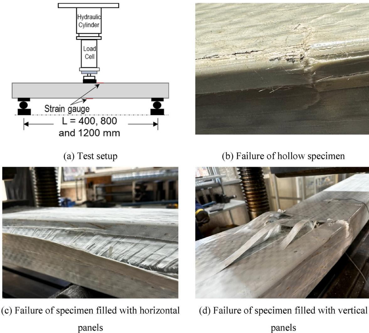
Fig. 7. Failure of beam specimens for different orientations of panels.
