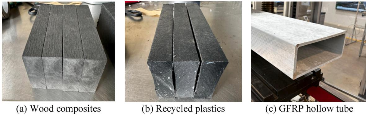
Fig. 2. Materials used in specimen preparation.
