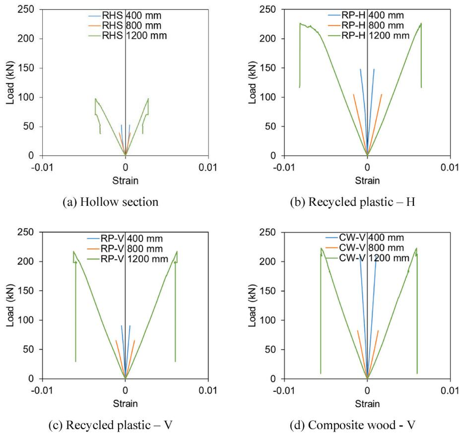
Fig. 8. Load-strain behaviour of different composite beams.
