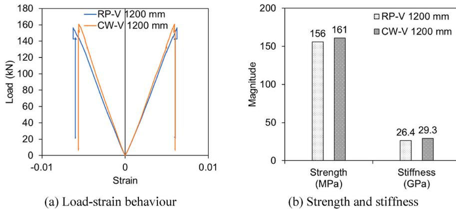
Fig. 11. Effect of in-fill panel material types.
