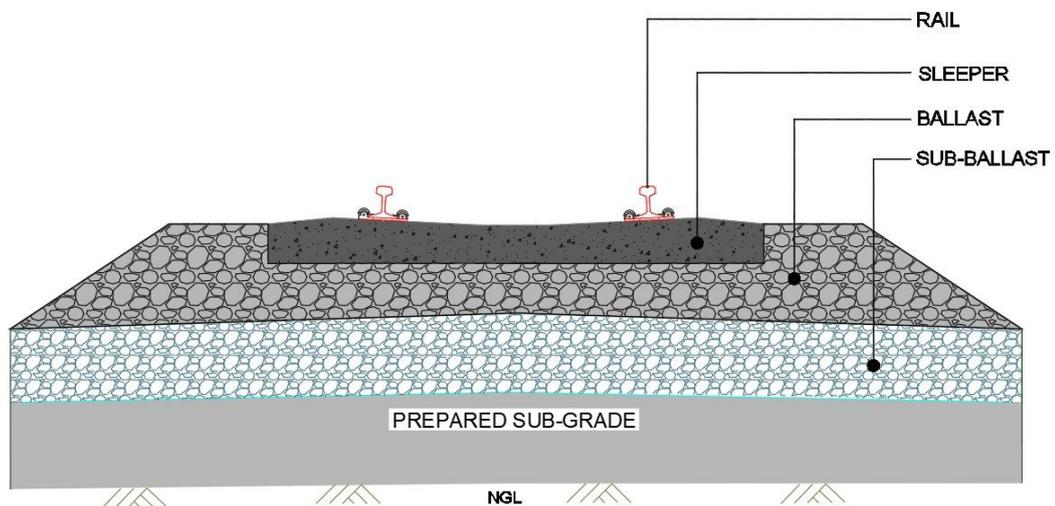
Figure 1: Basic components of typical railway track
