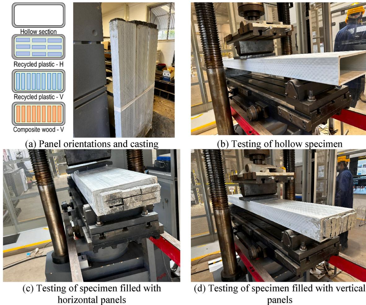
Fig. 4. Casting and testing of specimens.
