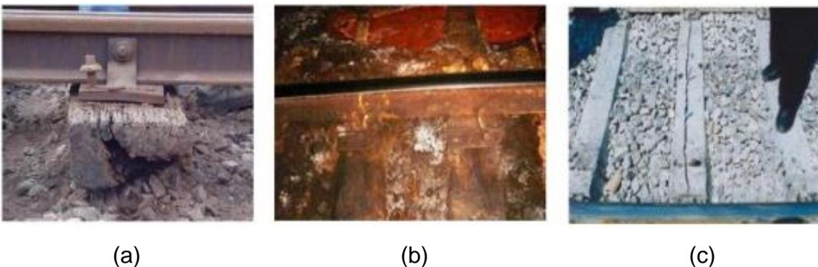
Figure 2: Premature failure of traditional sleepers (Ferdous & Manalo, 2014; Manalo et al., 2010): (a) timber (b) steel and (c) concrete
