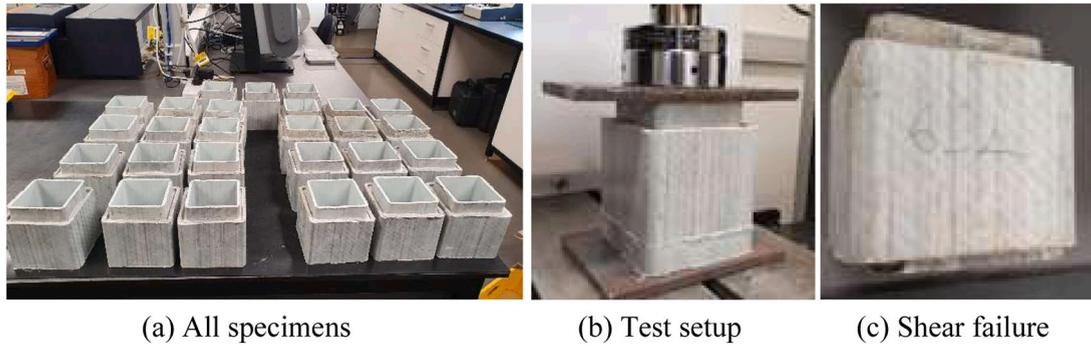
Fig. 2. Specimens, test set-up and failure mode.
