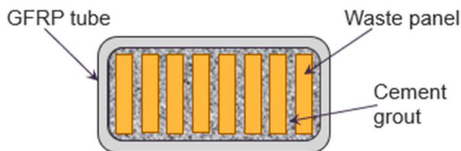
Fig. 1. Concept of composite railway sleepers.
