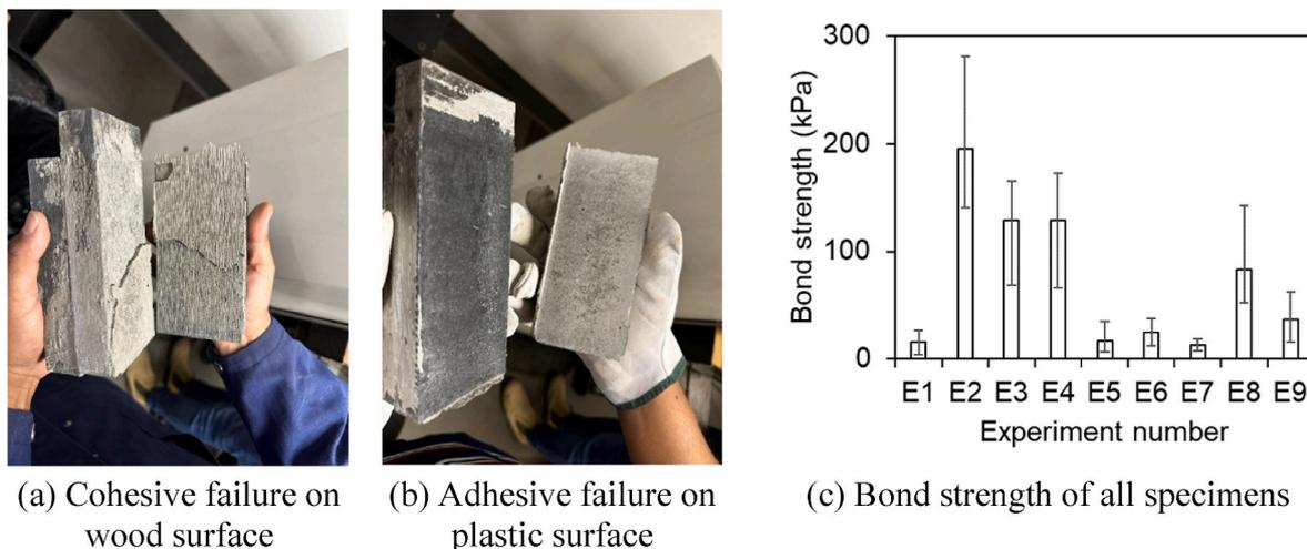
Fig. 5. Failure and strength behaviour of wood composite and recycled plastic panels.
