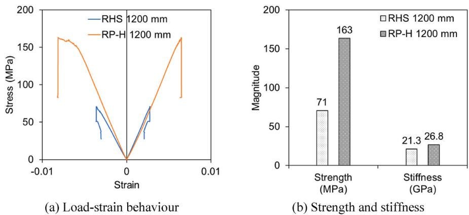
Fig. 9. Effect of filling hollow tubes.
