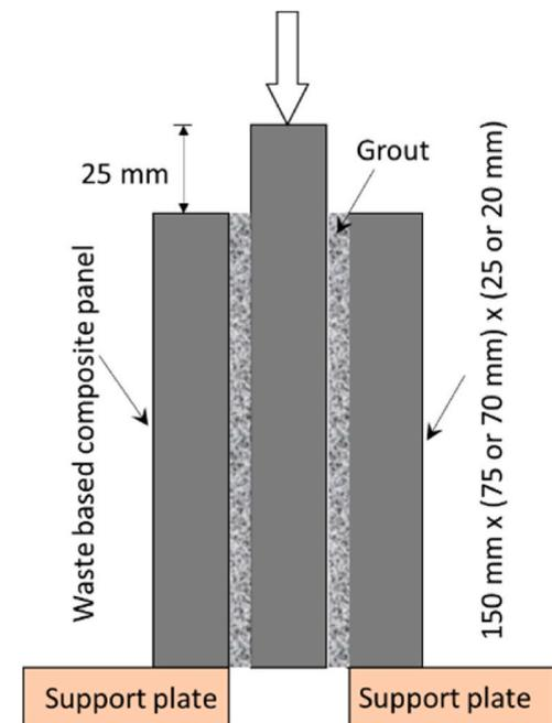
(a) Schematic diagram of bond test
