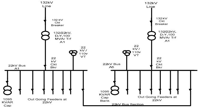
Fig. 5. SLD of a 132/22kV substation.
