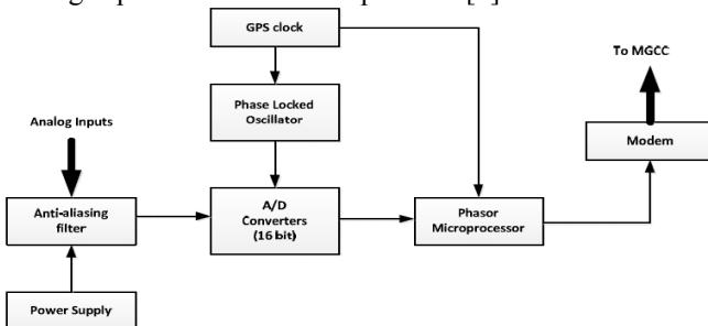
Fig. 1. Process block diagram of a PMU [1].
