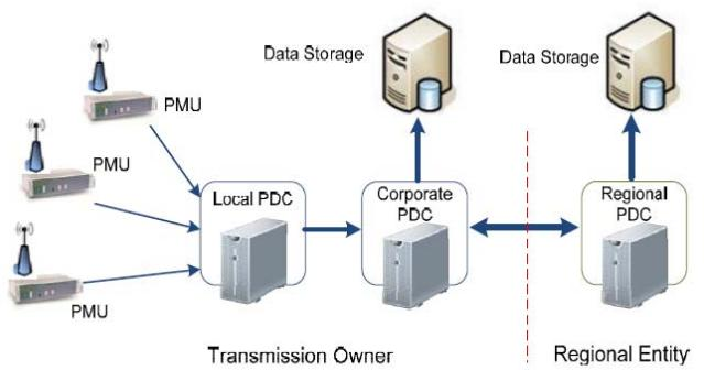
Fig. 3. PMU and PDC set up in wide area network [6].
