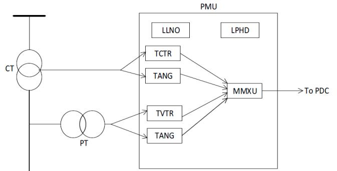
Fig. 2. PMU connectivity in a substation [1].
