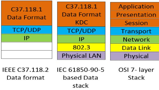
Fig. 4. IEC 61850-90-5 vs. IEEE and OS-7 Layer Stack [1].
