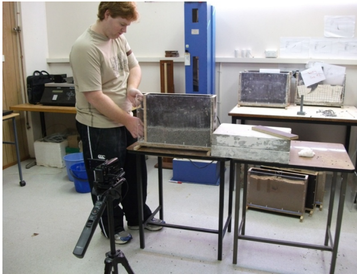
Figure 5: The setup for capturing videos for PIV analysis.
