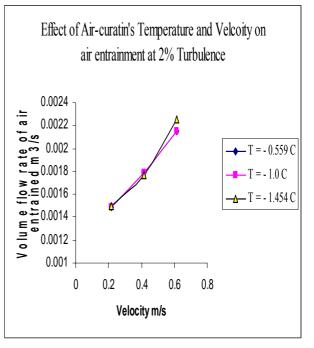
Figure (9) Effect of air-curtain's temperature& velocity on air entrainment at 2% turbulence
