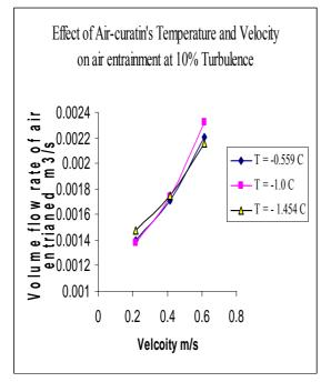
Figure (8) Effect of air-curtain's temperature& velocity on air entrainment at 10% turbulence
