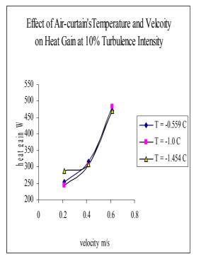
Figure (6) Effect of air-curtain's temperature and velocity on heat gain at 10% turbulence
