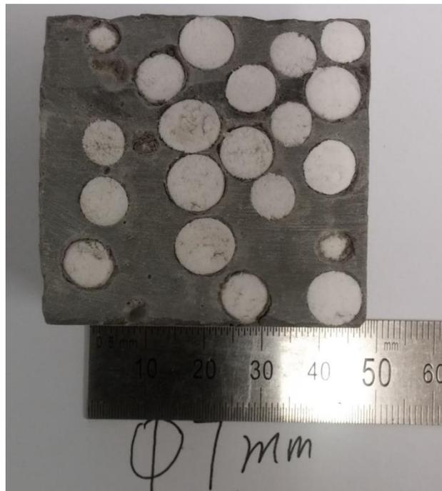
Figure 5. 4 EPS beads distribution of  $r=3.5\text{mm}$ ,  $V_f = 30\%$ ,  $S=41\%$ ; a) simulated EPS beads distribution; b) real experimental image
