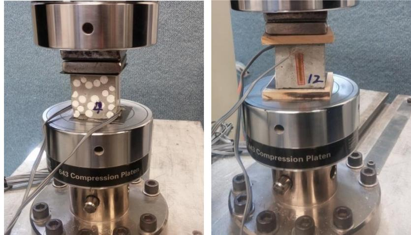
Figure 3. 4 Strain gauges on the sample
