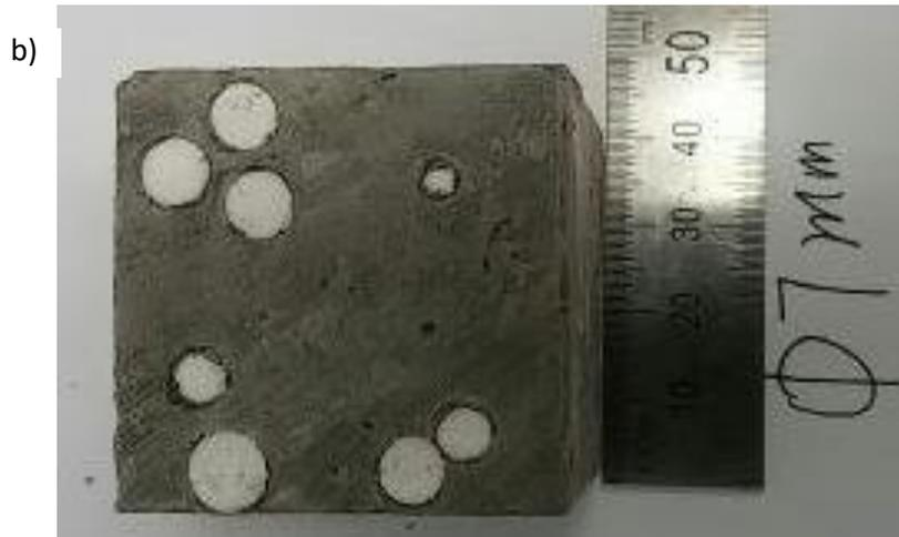
Figure 5. 2 Representation of EPS beads distribution of  $r=3.5\text{mm}$ ,  $V_f = 5\%$ ,  $s=16\%$ ; a) simulated EPS beads distribution; b) experimental images
