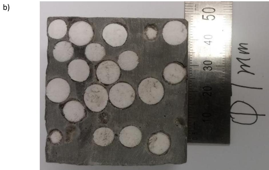
Figure 5.3 EPS beads distribution of  $r=3.5\text{mm}$ ,  $V_f = 20\%$ ,  $S=34\%$ ; a) simulated EPS beads distribution; b) real experimental image
