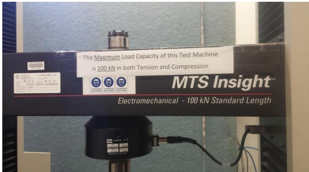
Figure 3. 2 Compressive strength test machine
