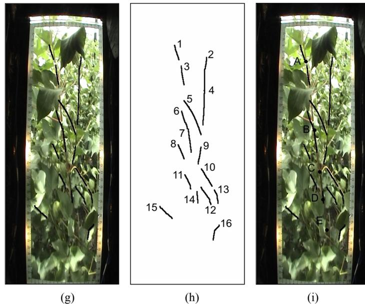
**Fig. 2. cont.** Image processing steps: (g) Steger lines superimposed on (a); (h) Labeled Steger lines; and (i) Steger lines and candidate nodes superimposed on (a), where A, B, C, D and E are node predictions based on the extrapolation of lines 1, 6, 8, 9, 11 and 15 from (h) onto the main stem respectively.
