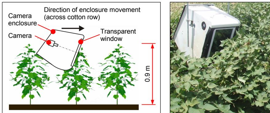
Fig. 1. Diagram and photo of moving image capture apparatus
