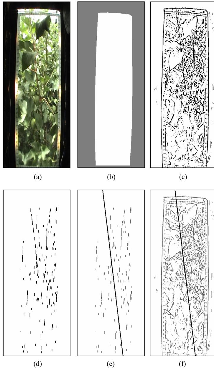
**Fig. 2.** Image processing steps: (a) Sample deinterlaced image captured from enclosure; (b) Mask for window area; (c) Adaptive threshold; (d) Morphological opening; (e) Hough transform line superimposed on (d); and (f) Hough transform line superimposed on (c).
