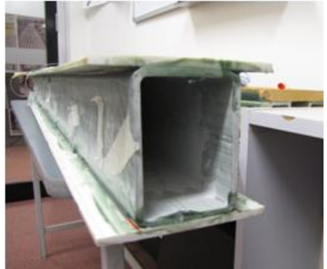
Figure 7. Prototype I beam with embedded FBG sensors
