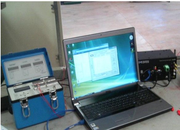
Figure 5. Usual experimental set up FBG readings
