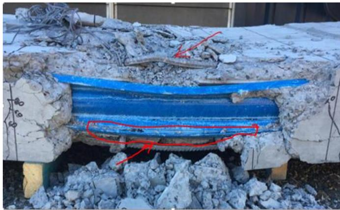
Figure 4. 29 Compressive steel buckling failure (S4).
