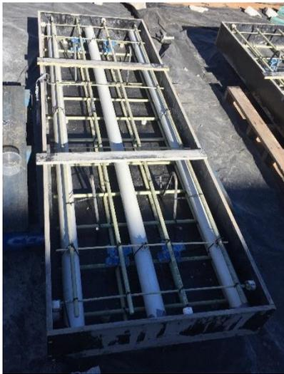
(a) Slab S2 with PVC pipes before casting
