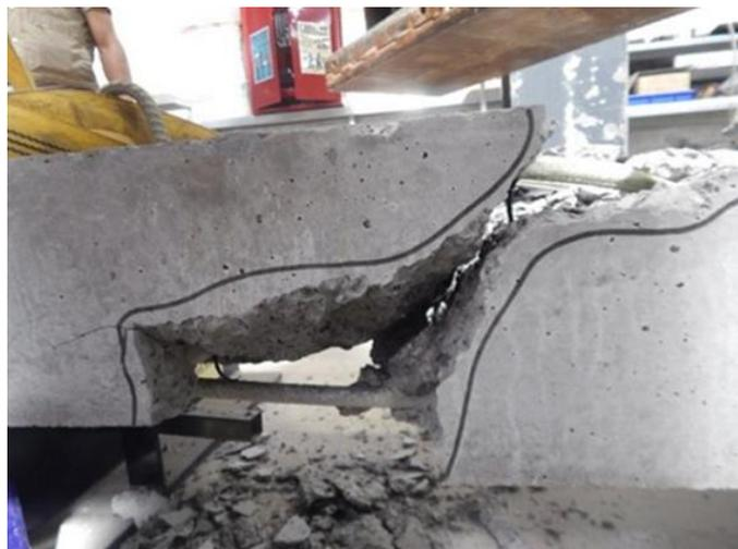
Figure 4.4 Final failure (S1).
