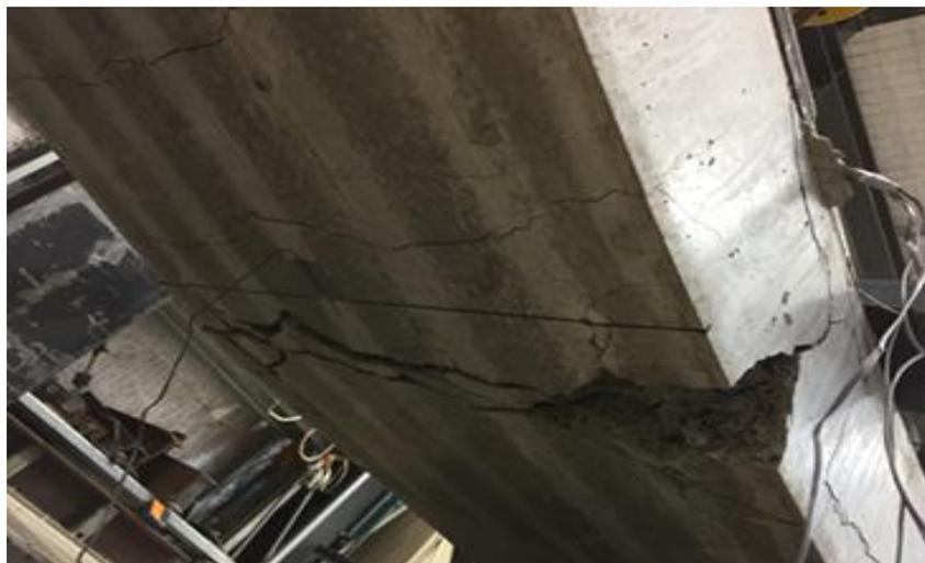
(b) Hollow slab with CRS provided perfect failure behaviour as shown in the bottom slab.
