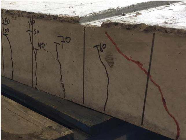
Figure 4.9 Cracks propagated upwards (S2).
