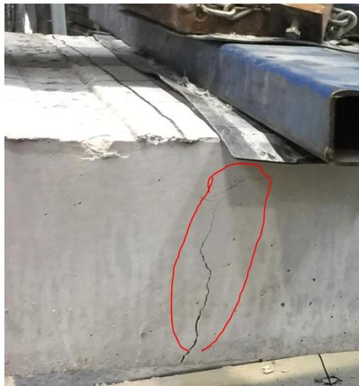
Figure 4.3 Crack propagated close to the point load (S1).
