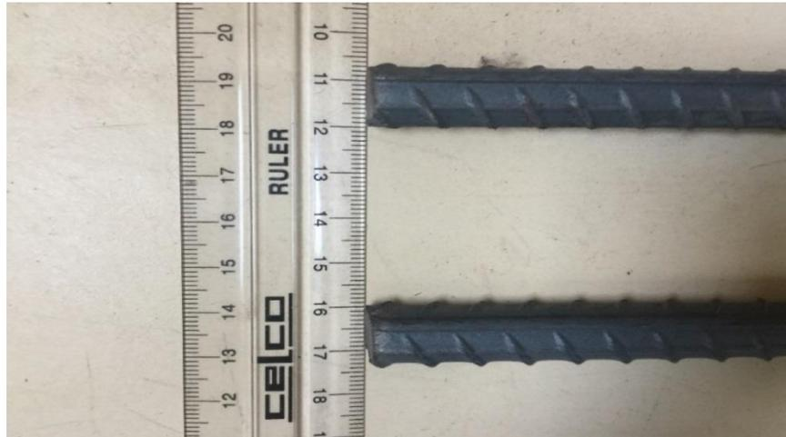
Figure 3.4 Steel bars (12 mm diameter).
