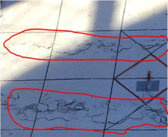
Figure 4. 27 Cracks initiation in the top concrete (S4).
