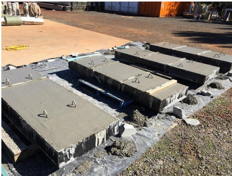
Figure 3.10 Specimens after casting.
