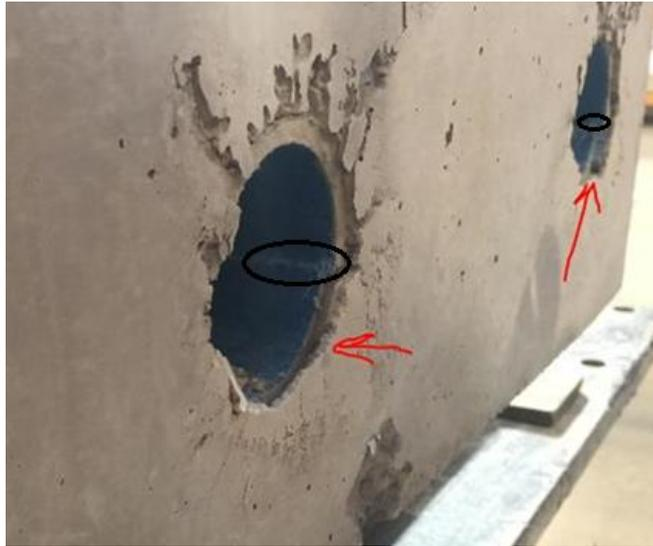
Figure 4. 20 CRS debonding (S3).
