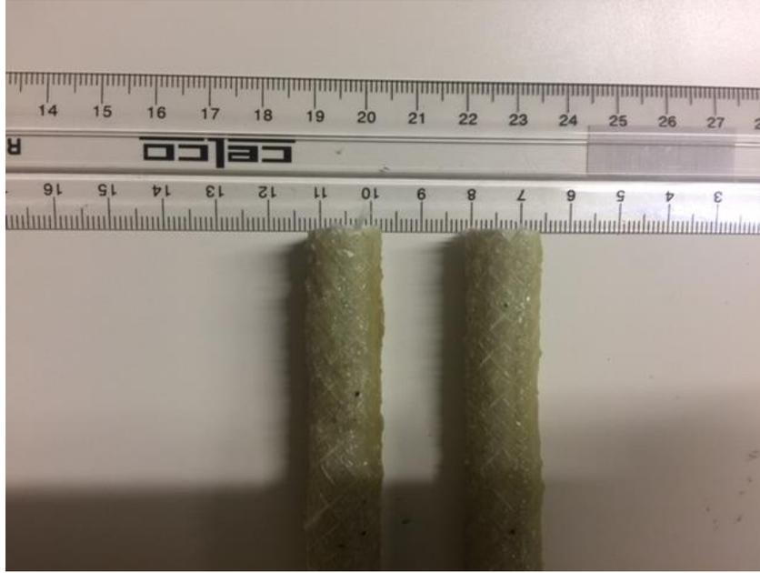
Figure 3.3 GFRP bars (12 mm diameter).
