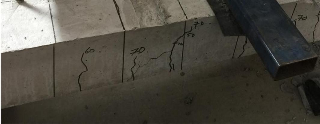
Figure 4.2 Cracks propagated upwards (S1).
