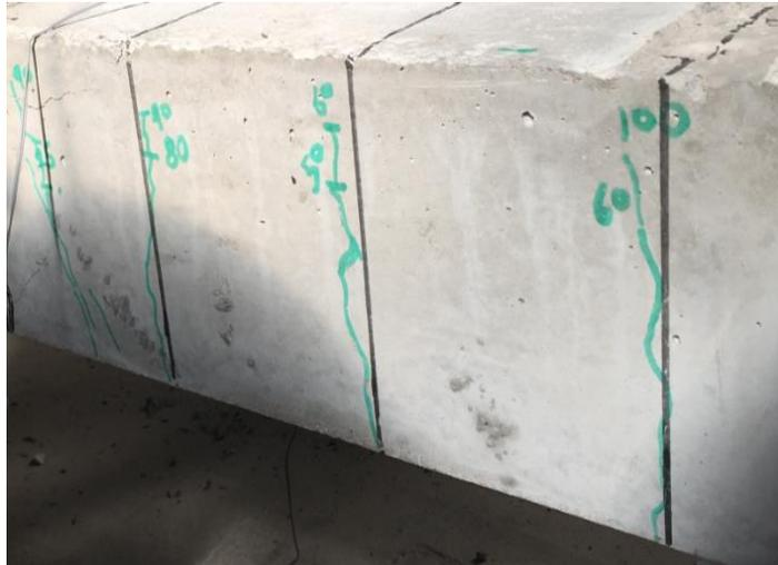
Figure 4. 16 Initiation of horizontal cracks (S3).
