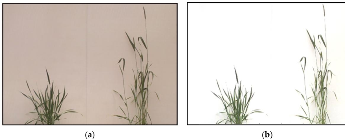
Figure 9. Output of RGB images after (a) gradient correction and (b) illumination correction.
