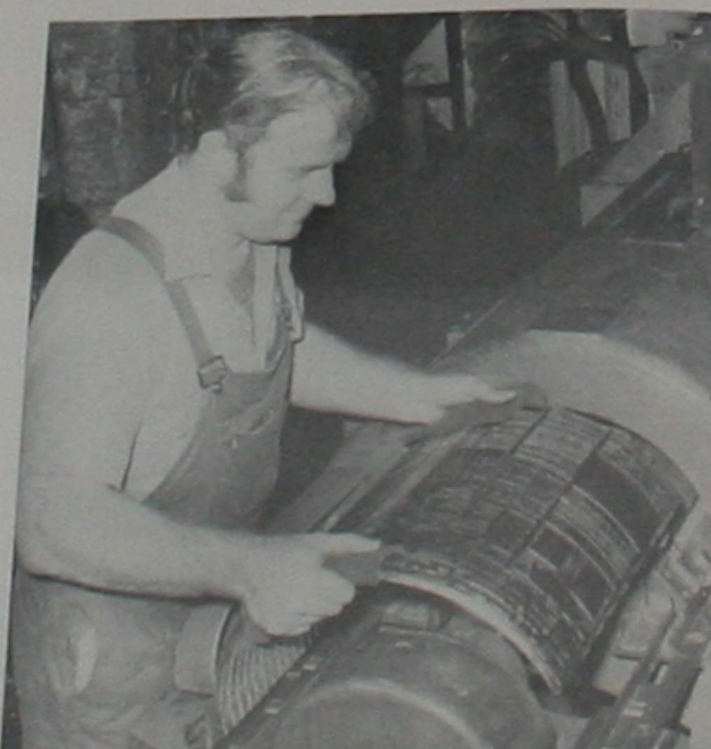
• The press plate, made from the matrice, is trimmed
