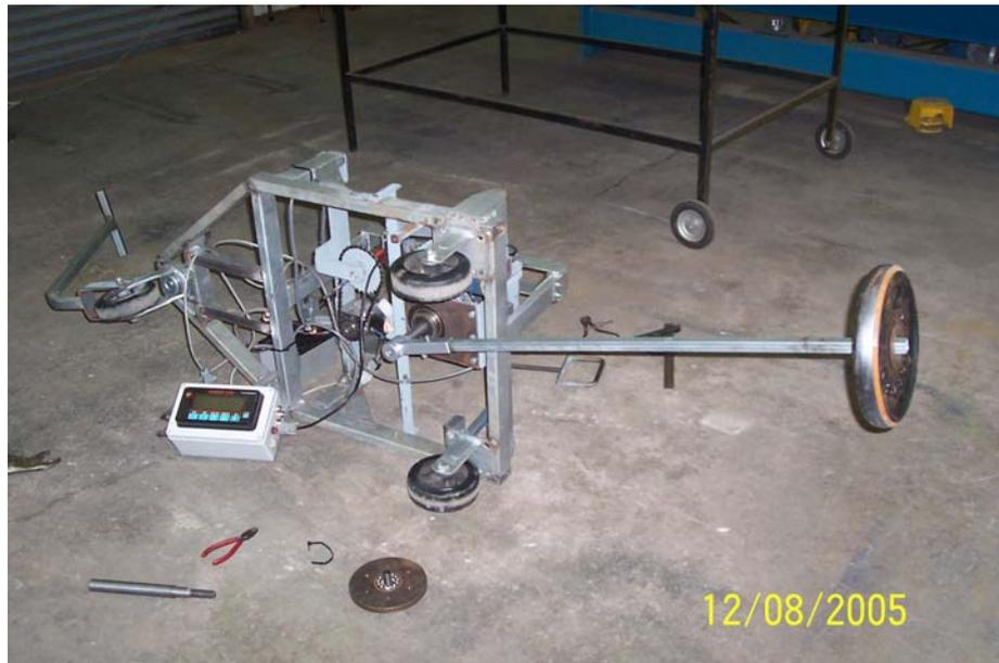
**Figure 6.3 Calibration weight and loading arm**
