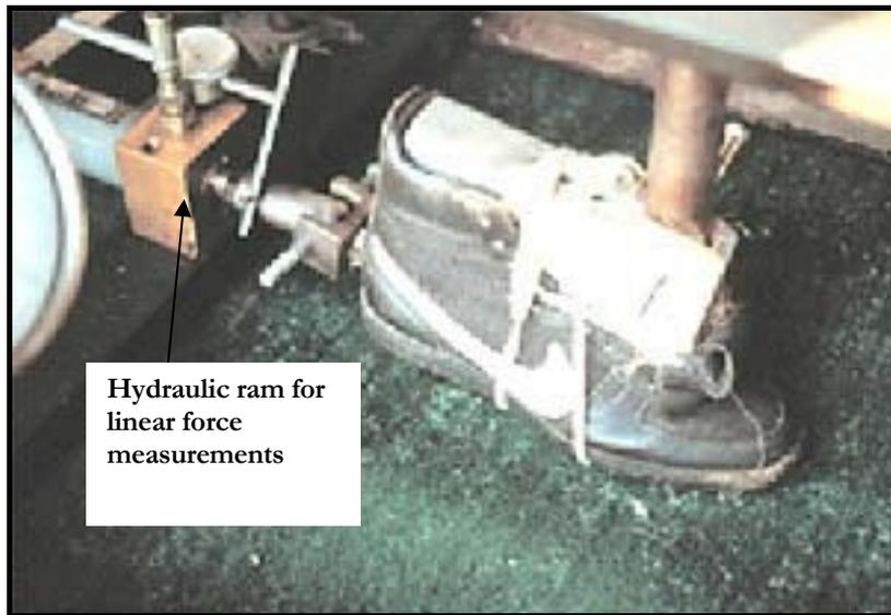
Figure 3.3 Pennfoot linear operation
