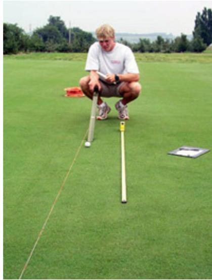
**Figure 2.1 Basic rolling resistance method using a stimpmeter**
