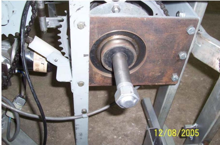
**Figure 6.4 Calibration loading nut**
