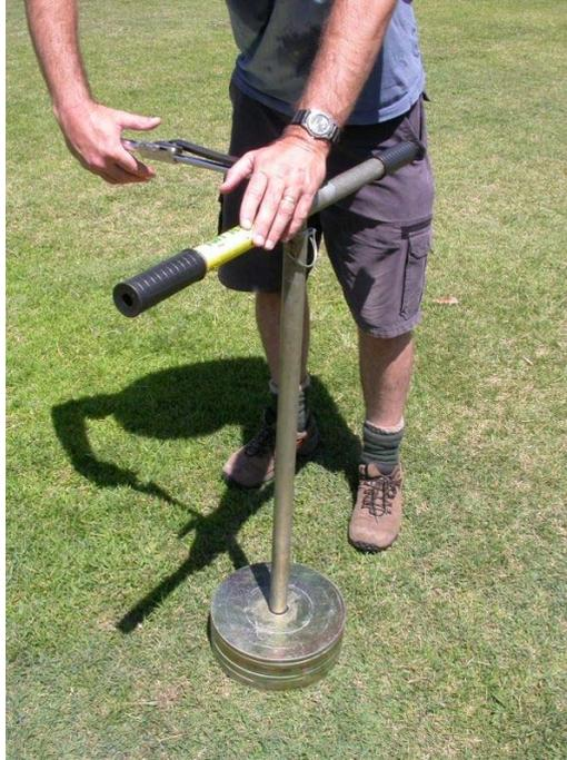
**Figure 2.3 Manual traction measuring device sold in Australia
