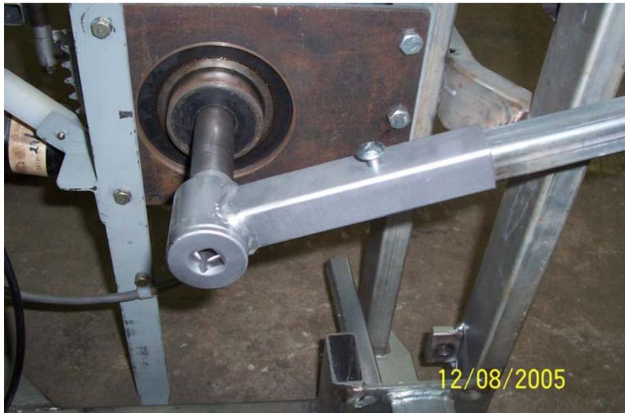
**Figure 6.5 Calibration loading arm attachment**
