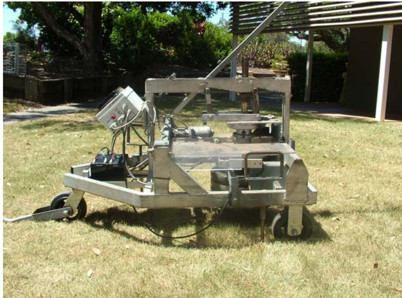
(b) Final prototype with lifting parallelogram
