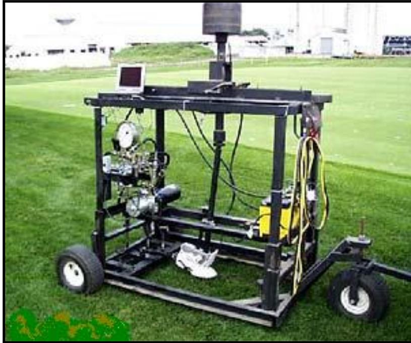
Figure 3.2 McNitt's "Pennfoot" device for measuring traction.
