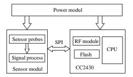
Figure 4. Structure ZigBee sensor node module
