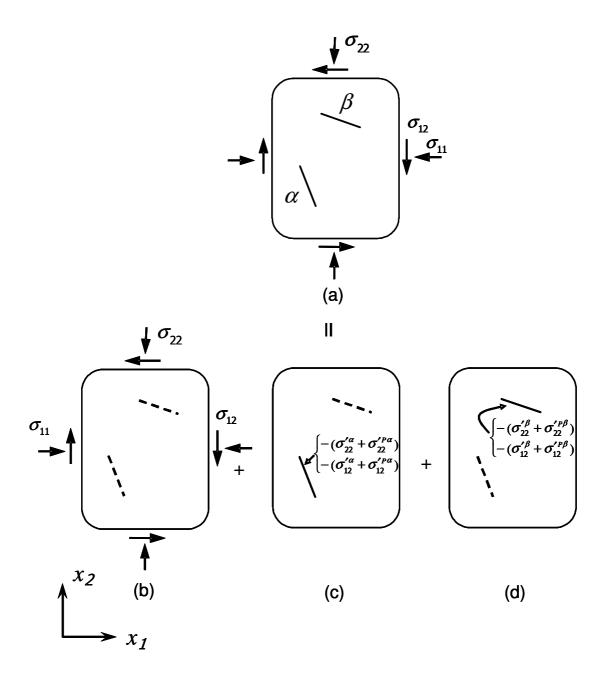
Fig. 3. Decomposition of (a) the original problem into (b) the homogeneous problem and (c) and (d) two sub-problems
