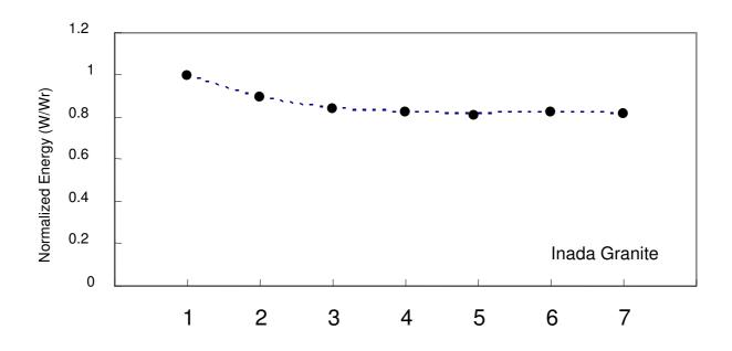
Fig. 5. Normalized energy for the meshes with different number of elements and nodes (Inada Granite)
