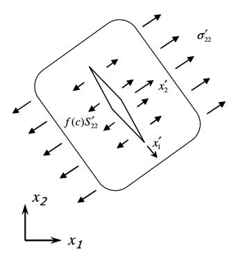
Fig. 2. A single microcrack under local stresses
