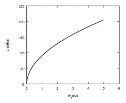
Fig. 7. Relationship between pressure p and strain energy Ws transferred to the surrounding
