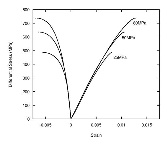
Fig. 4. Stress strain curves for Inada granite
