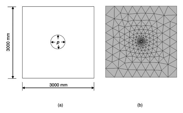
Figure 6. (a) A region with a hole inside under pressure of p (not scaled) (b) Finite element mesh
