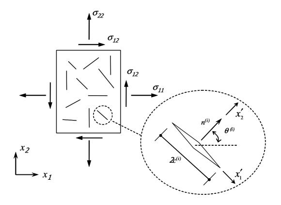
Fig. 1. Rock material containing numerous microcracks
