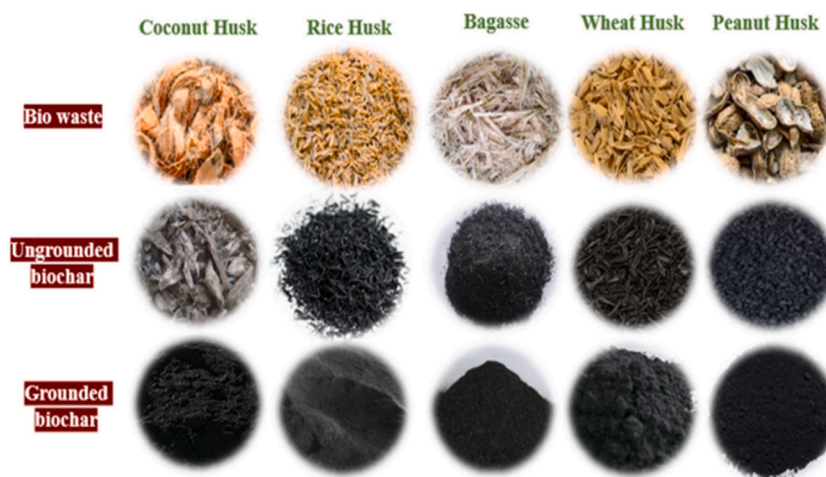
Fig. 4. Grounded and ungrounded biochar produced from raw biowastes through pyrolysis.
