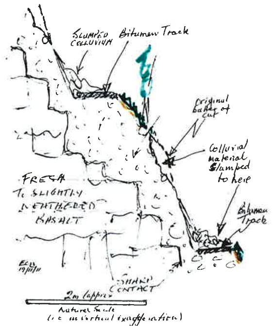
Figure 3 Effects of track construction on the geology on the Fantail Track
