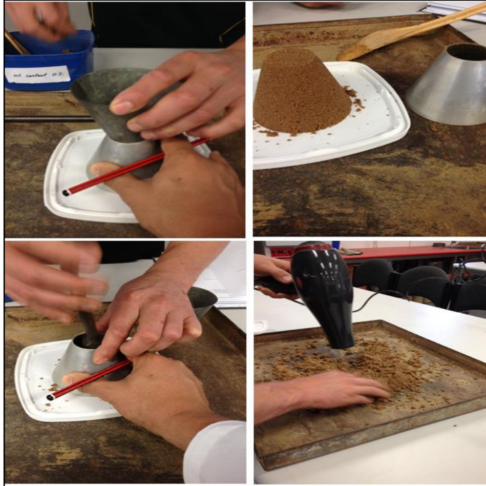
Figure 3.6 Procedure of water absorption test based on AS 1141.5
