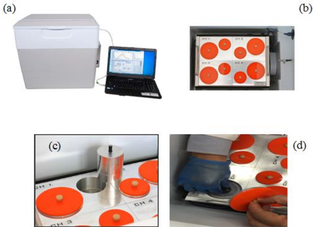
Figure 4.4 I-Cal isothermal calorimeter (I-Cal 4000)
