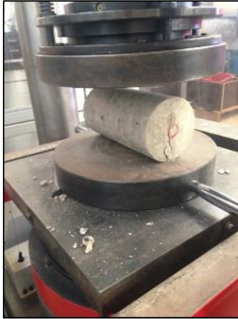
Figure 8.3 Splitting tensile test using SANS machine
