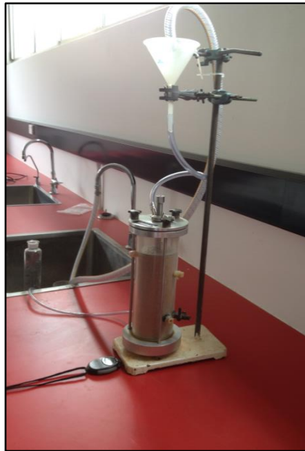
Figure 3.9 Constant-head permeability test
