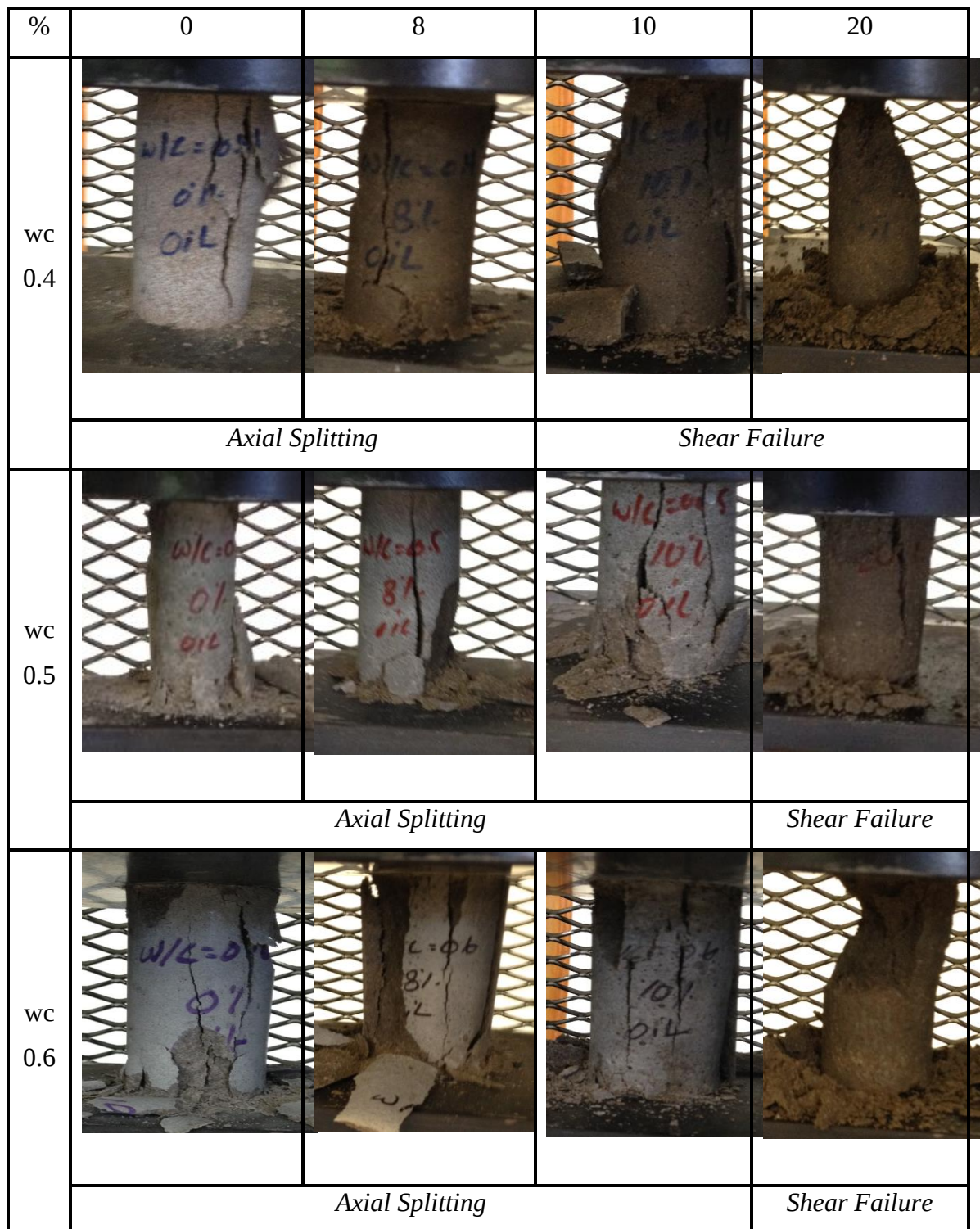
Figure 5.3 Failure mode of different w/c ration and different crude oil content
