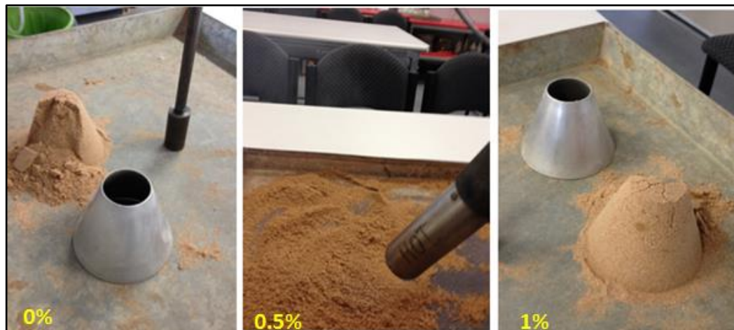
Figure 3.11 Water absorption test for 0, 0.5 and 1% oil-contaminated sand.
