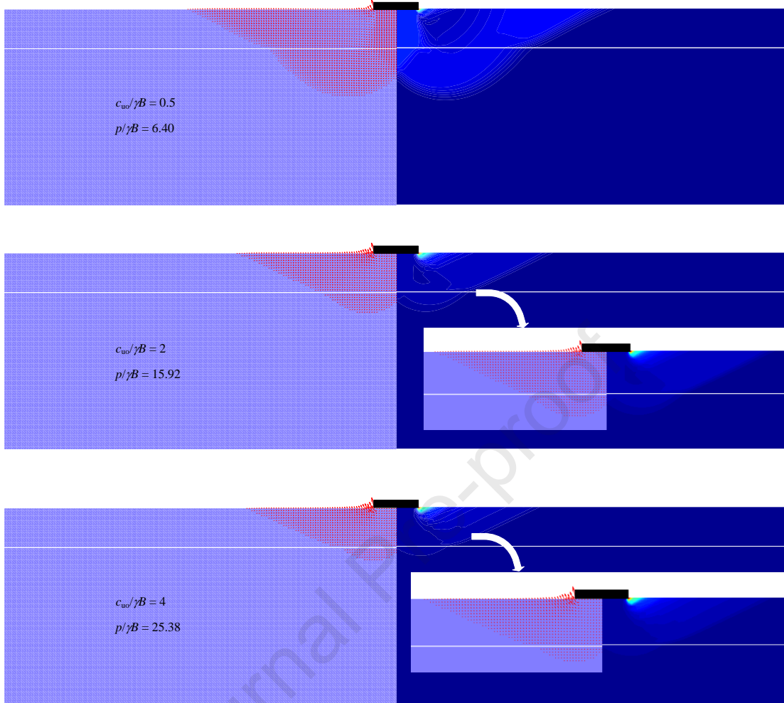
Fig. 11. Effect of c_{u0}/\gamma B on failure mechanisms ( H_1/B = 1 , q/\gamma B = 0 , \varphi' = 40^\circ ).
