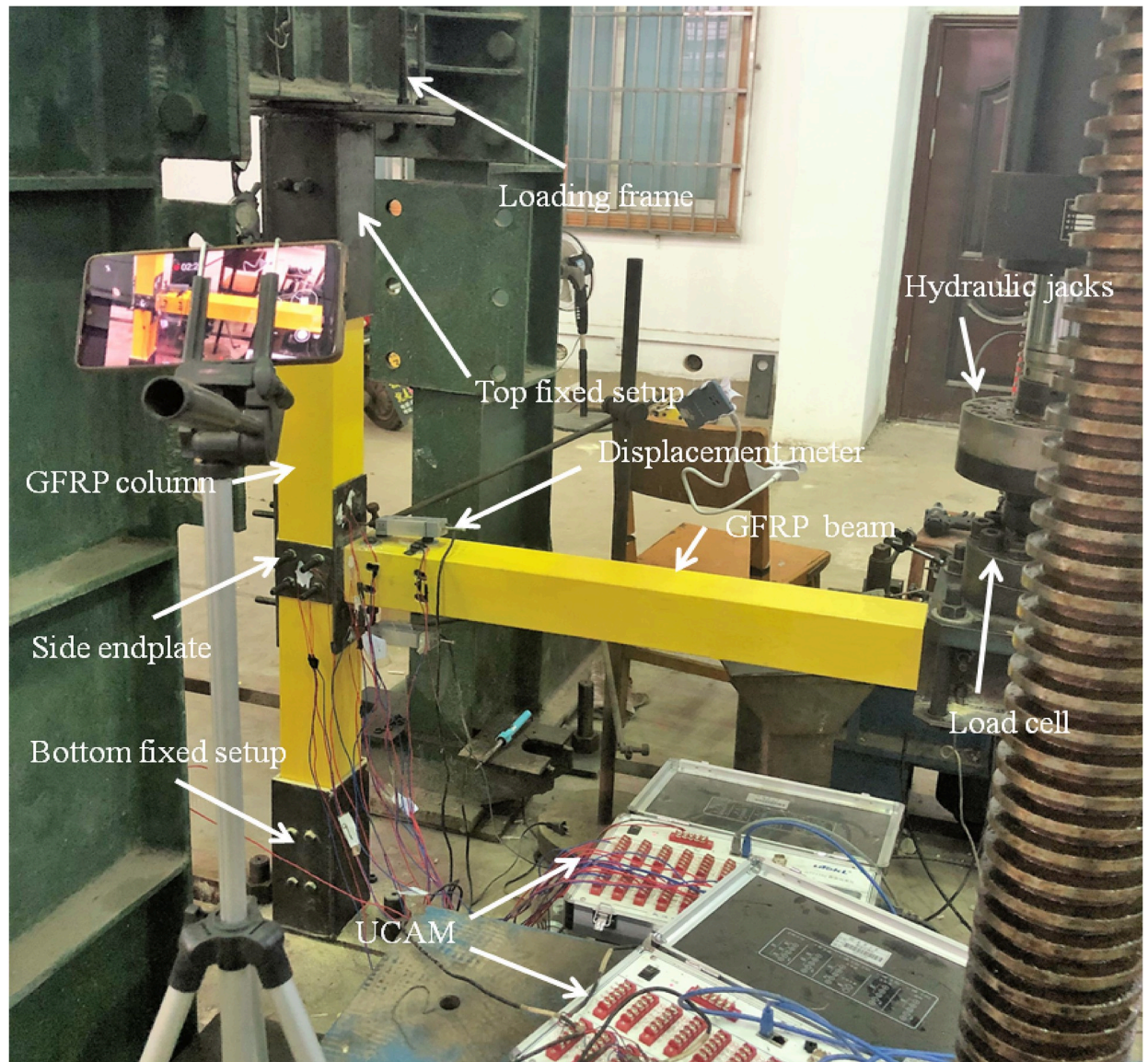
Fig 3. Experimental set-up for specimens.
