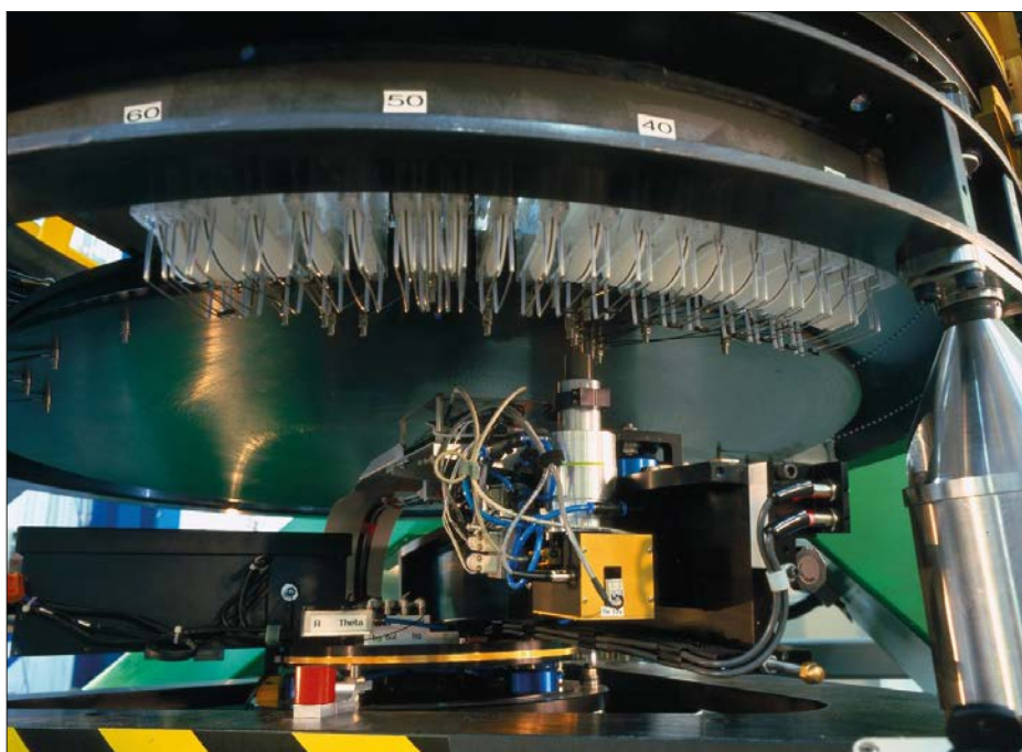
8 AAO gets its own back. The OzPoz fibre positioner was built by the AAO for the VLT's FLAMES multi-object spectrograph. This early example of Australian equipment on overseas facilities is likely to be repeated under the new strategic partnership. (ESO)
