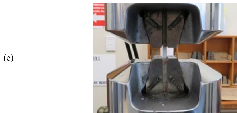
Fig. 4. Details of compression coupons (mm) (a) square tubes (S1), (b) square tubes (S2), (c) circular tubes, and (d) compression coupons of FRP tubes and (e) set-up of the compression test.
