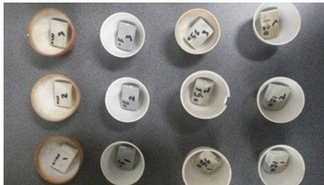
Fig. 2. Coupon specimens for burnout test.
