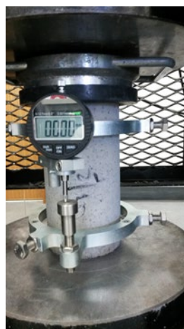
Figure 3.2 Measurement of longitudinal deformation
