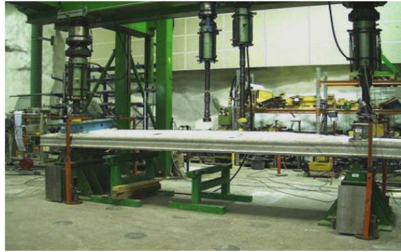
Figure A.3. Torsion test setup for hollow concrete plank (Pajari 2004; Derkowski & Surma 2015)
